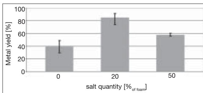
Fig. 5: Metal yield in dependence from salt quantity without  $\text{CaF}_2$  addition
