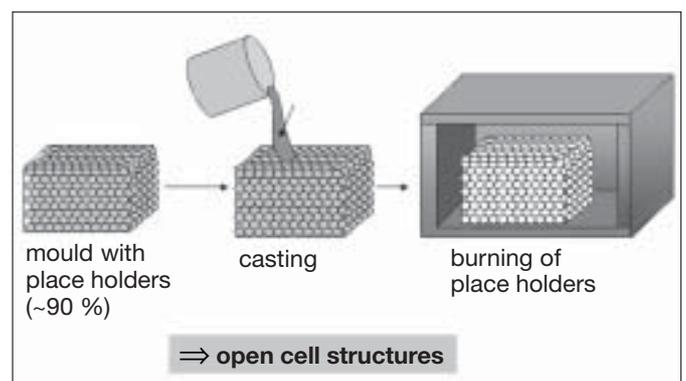
Fig. 2: Diagram of foam production by casting processes
