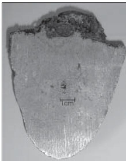
Fig. 7: Aluminium ingot with pores
