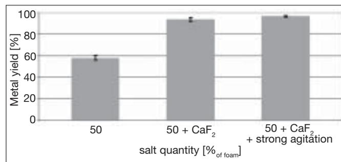
Fig. 6: Metal yield in dependence from  $\text{CaF}_2$  addition and agitating conditions
