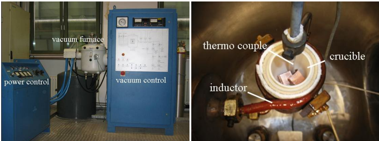
Figure 8: Induction furnace with controls (left) and construction inside furnace (right)
