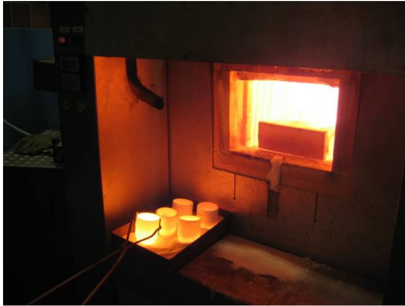
Figure 11: resistant heated furnace for kinetic trials
