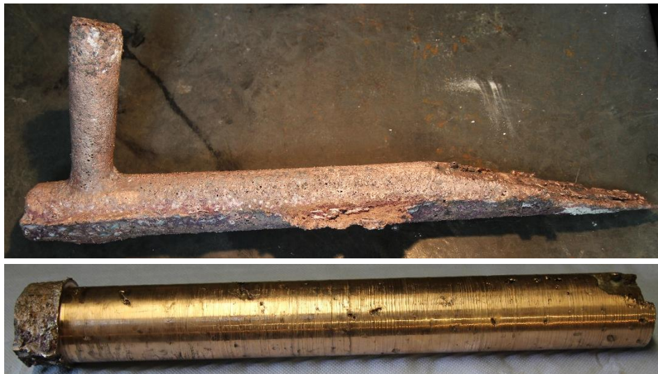
Figure 6: Metal product of ATR inline casting (top) and electrode prepared for VAR (bottom)
