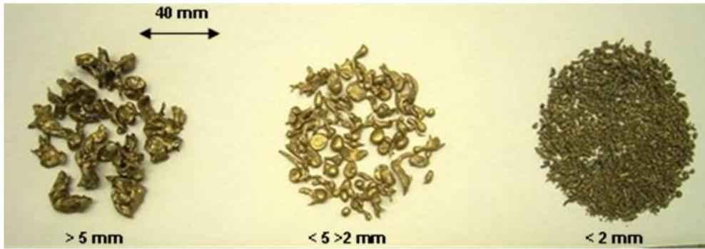
Fig. 2: A view of the different anode particle sizes (20 g each sample)
