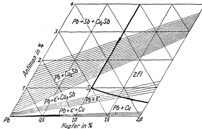
Figure 8: Lead corner at the Pb-Cu-Sb phase diagram after homogenisation at 20 - 30 °C below solidification temperature [11]
