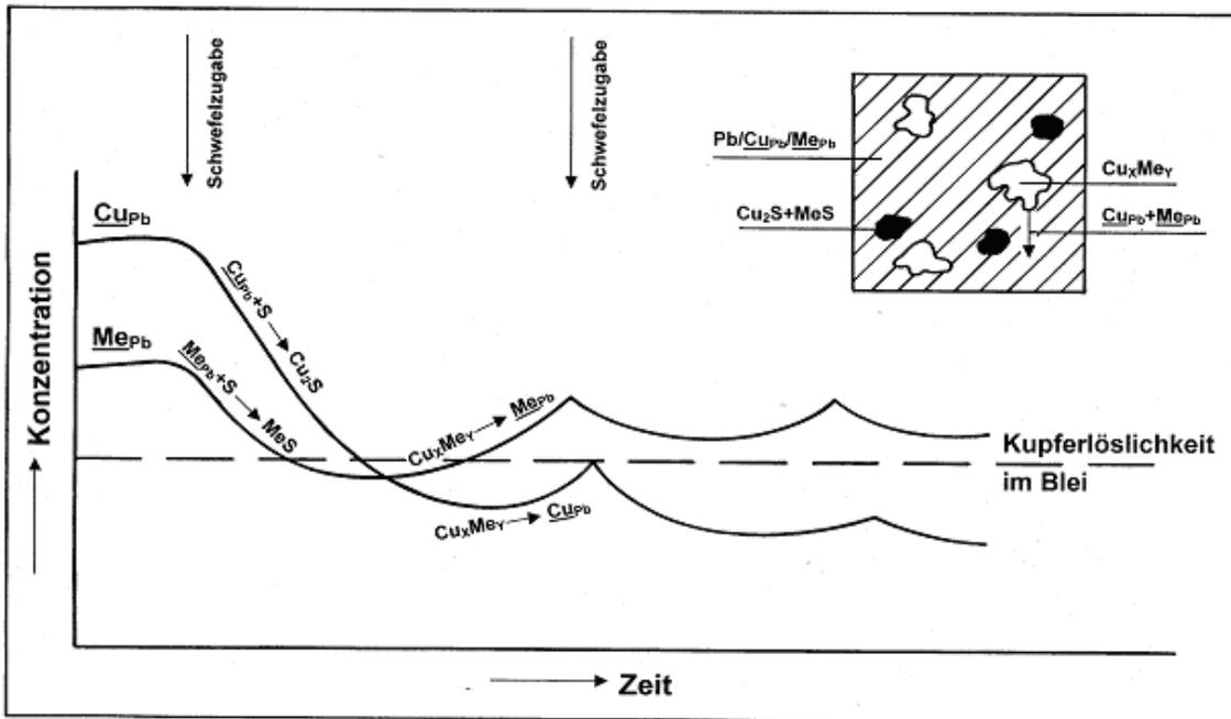
Figure 20: Schematic illustration of proposal mechanism for copper removal
