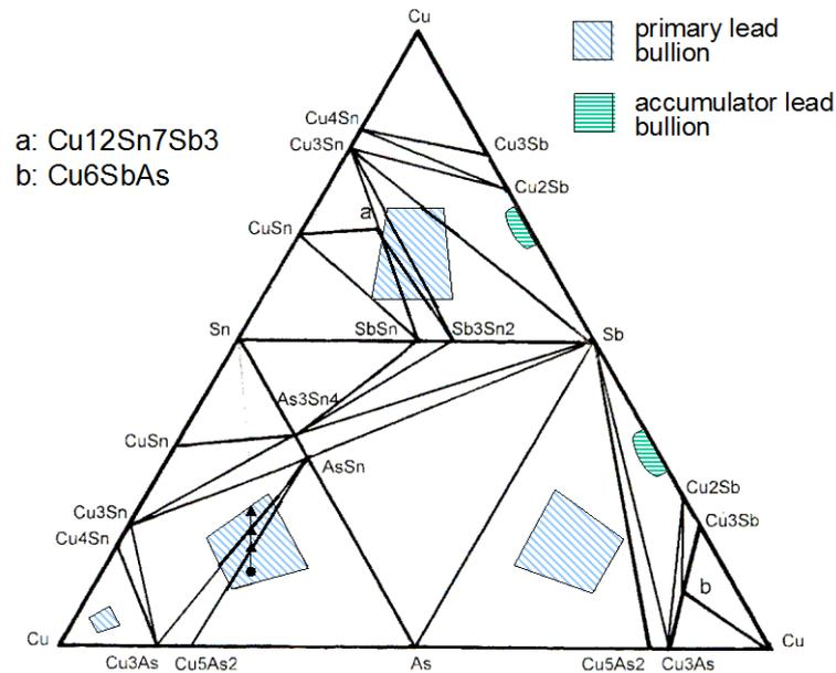
Figure 9 : Triangulation of the system Cu-As-Sb-Sn
