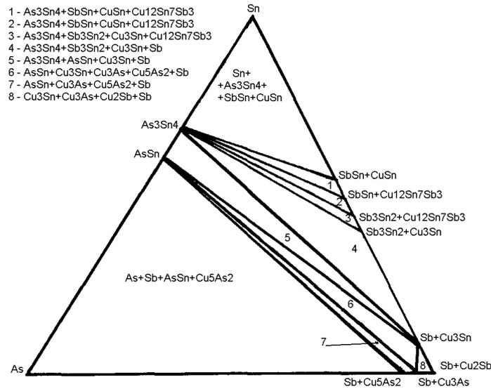
Figure 11: Polythermic cut As-Sn-Sb/Cu = 9,5 (bullion from battery recycling)
