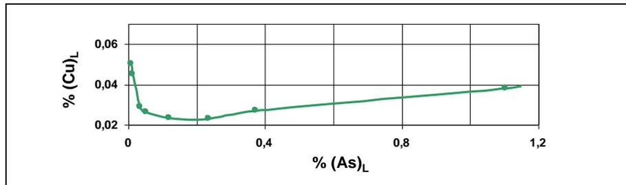
Figure 6: Pb-Cu-As-system; isotherm of Cu-solubility at 337 °C
