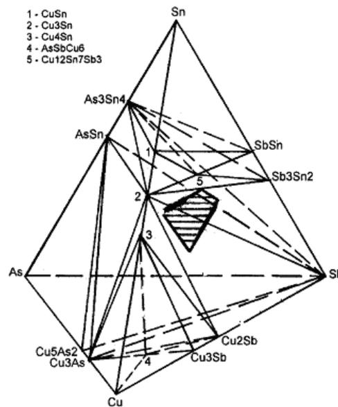
Figure 10: Tetraerdrat of the system Cu-Sb-As-Sn
