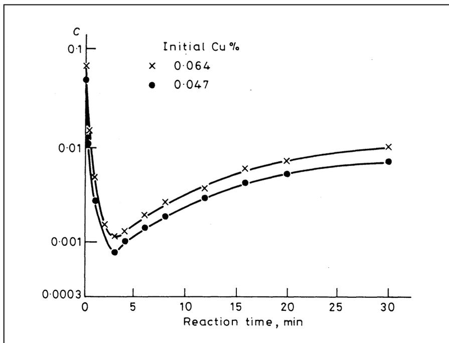
Figure 15: Kinetics of the copper removal from lead with sulphur [40]
