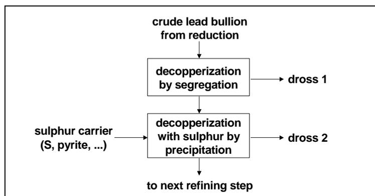
Figure 1: Scheme of the first refining step for crude lead
