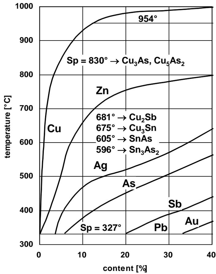
Figure 3: Equilibrium solubility of alloying elements in lead and melting points of relevant intermetallic phases [3]
