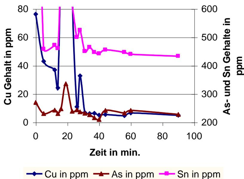
Figure 16: Kinetic curves of copper, tin and arsenic concentration by copper removal in lead with sulphur and pyrite (production samples)
