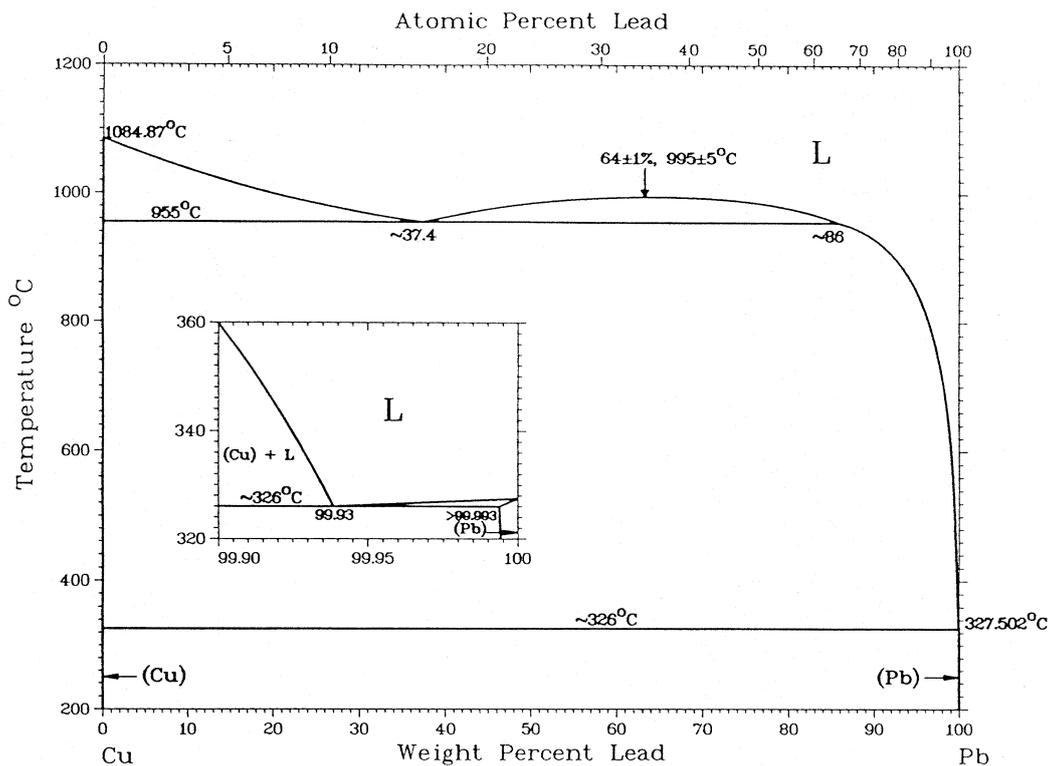
Figure 2: Binary-system Pb-Cu
