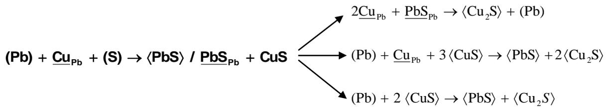
PbS and CuS as stable phases are formed when liquid or gaseous sulfur comes in contact with lead containing copper. CuS originates by a heterogeneous reaction between copper dissolved in lead and sulfur. It is there produced where sulfur is in a local surplus. According to the reactions (4) and (5) CuS contributes to a further decopperization [1,35].
