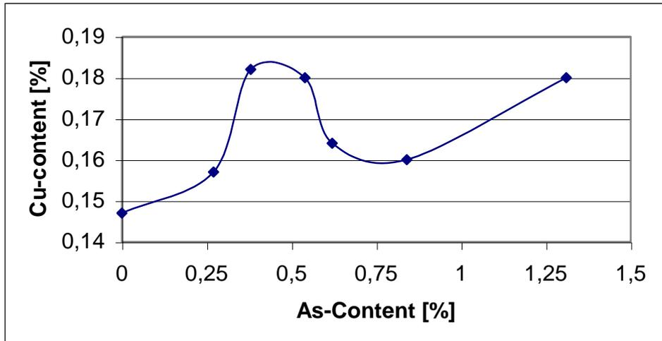
Figure 14: Influence of arsenic on the copper removal in the system Pb-Cu-Sb-As (single sulphur addition 100 %, Cu initial content from 0,30 to 0,50 %, Sb initial content 9 %)
