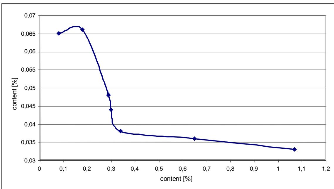
Figure 13: Influence of tin concentration on copper removal in Pb-Cu-Sn-Sn-melts at 285 °C (single sulphur addition 100 % related to Cu<sub>2</sub>S, Cu initial content 0.15 to 0.30 %, Sb initial content 9.0 %) [12]
