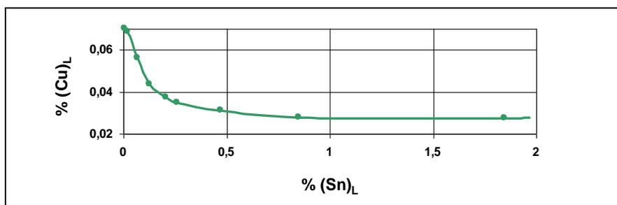
Figure 5: Pb-Cu-Sn-system; isotherm of Cu-solubility at 337 °C
