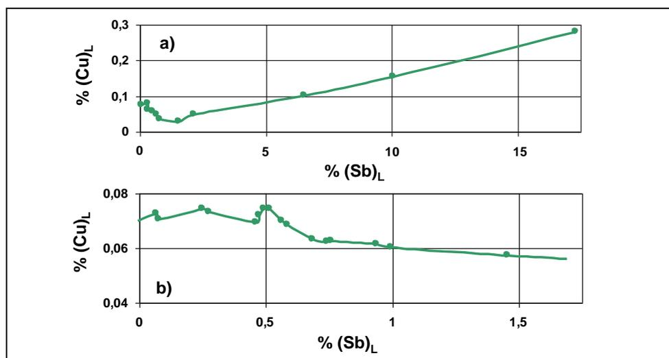
Figure 7: System Pb-Cu-Sb isothermal solubility of copper at 337 °C
