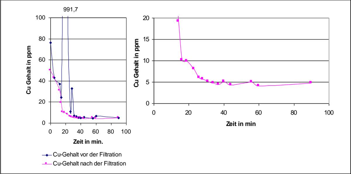
Figure 17: Copper concentration versus reactiontime
