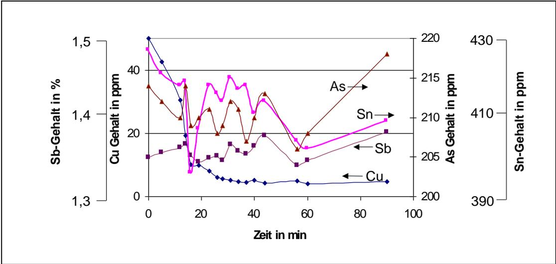
Figure 18: Concentration of copper, tin, arsenic and antimony during sulphur addition treatment (after sample filtration)
