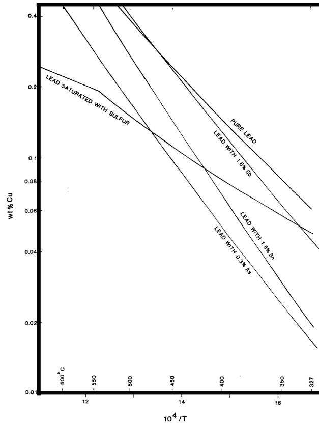
Figure 4: Solubility of copper in lead as a function of temperature in presence of third elements
