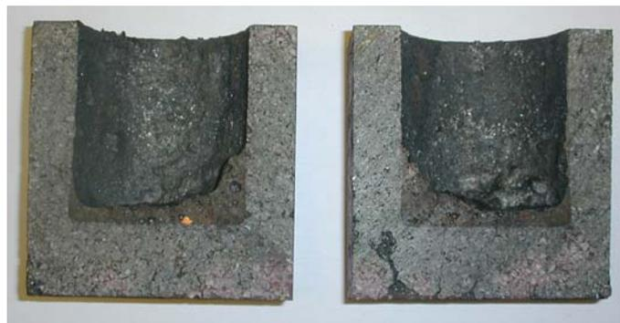
Figure 5: Slag-refractory interaction in chrome-corundum crucible.
