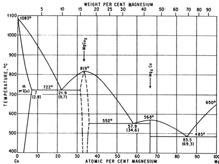
Figure 1: Copper-magnesium phase diagram [5].
