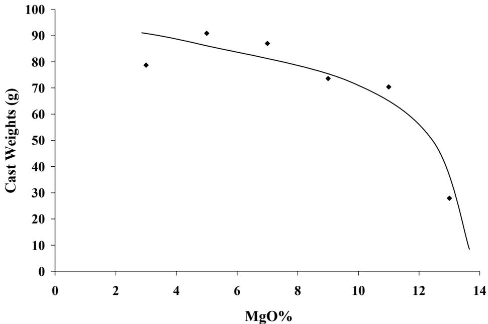
Figure 4. Cast weights vs. MgO content of the slag.
