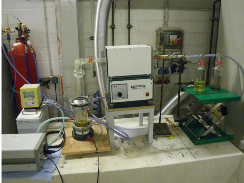
Fig. 2 Experimental setup for the USP-synthesis of gold nanoparticles at IME, RWTH Aachen
