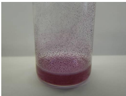
Figure 6: Precipitation of gold nanoparticles in water solution (Exp. 1)
