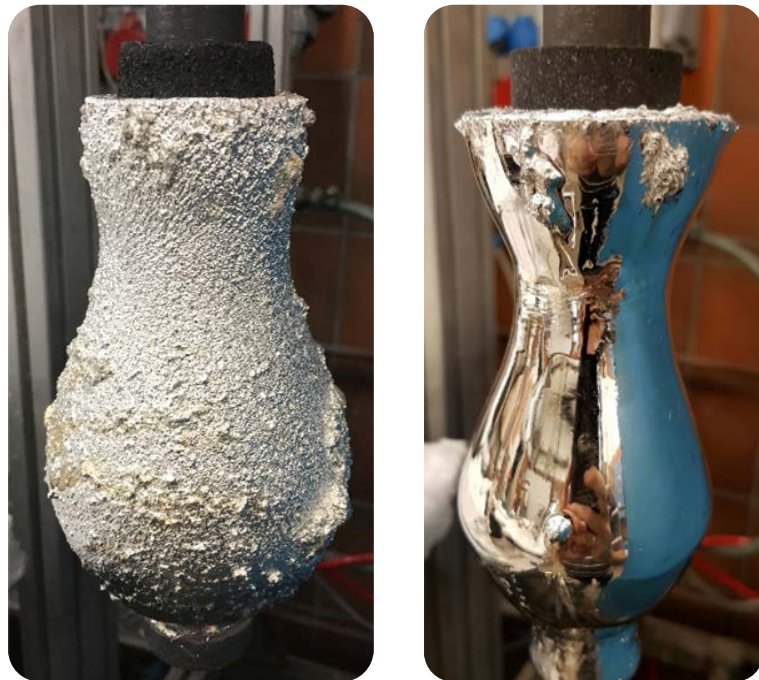
Figure 7. The difference on the crystallization surface between an experiment without (left) and with (right) rotation.
