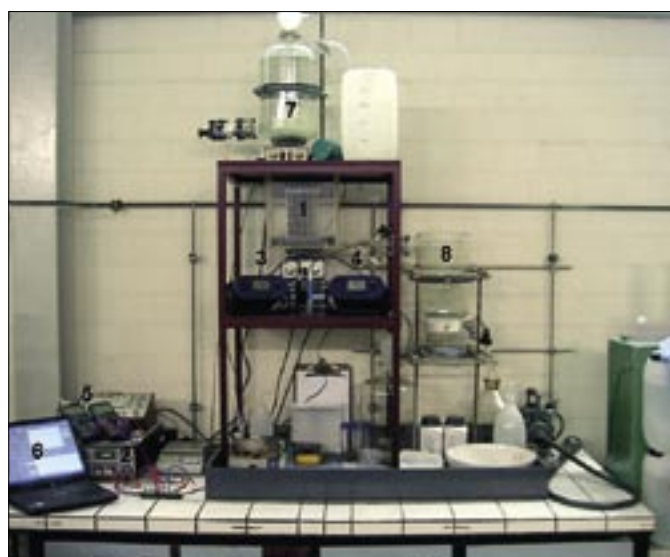
Fig. 5: Electrocoagulation system at IME RWTH-Aachen, Germany
