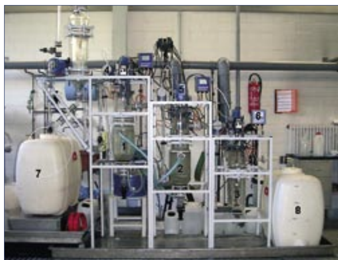
Fig. 7: Continuous 3 reactor precipitation line at IME RWTH-Aachen, Germany
