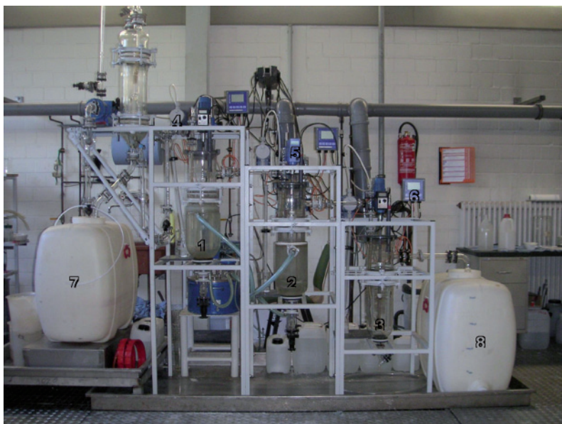
Fig. 4: Continuous 3 reactor precipitation line at IME RWTH-Aachen, Germany
