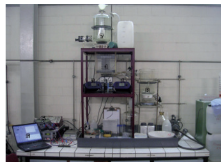
Fig. 6: Electrocoagulation system at IME RWTH-Aachen, Germany
