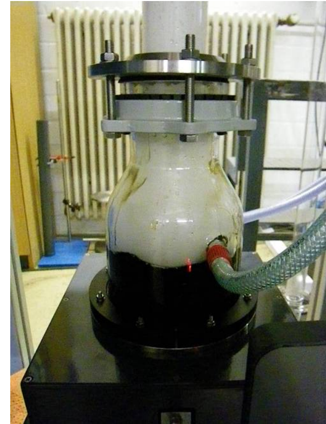
USP production of aerosol with 3 ultrasonic transducer (IME RWTH Aachen)
