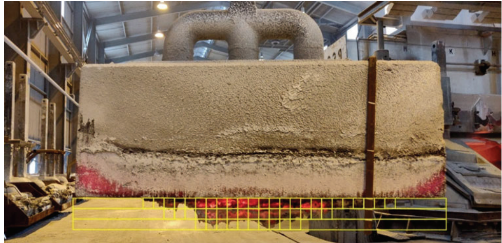
Fig. 2 5 cm by 5 cm grid for measurement of thickness and position of frozen bath layer underneath anode after the experiment's duration, Cell 239, anode K/8; Carbon Dust index 1/2, no pacman, anode set too low, duration 2 h. (Color figure online)
