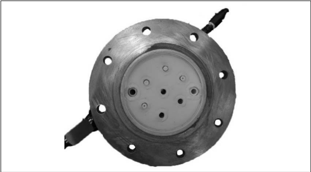
Figure 1: Lid of the electrolysis cell with white powdery condensate
