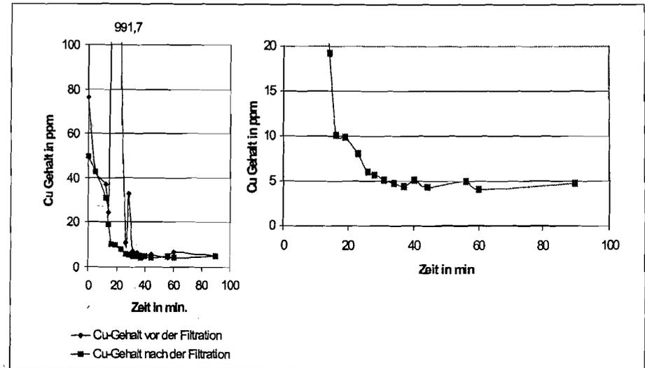
Figure 17: Copper concentration versus reactiontime
