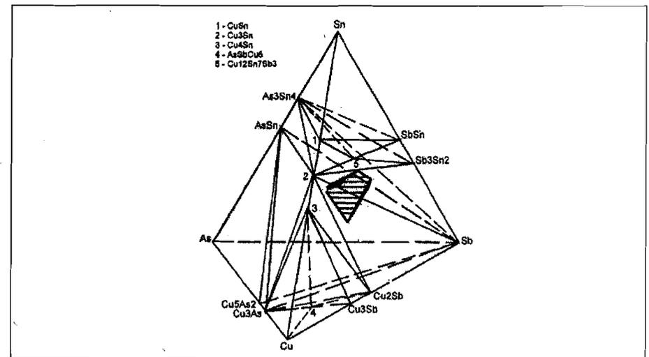
Figure 10: Tetrahedration of the system Cu-Sb-As-Sn
