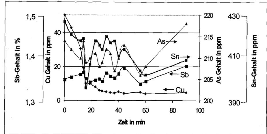
Figure 18: Concentration of copper, tin, arsenic and antimony during sulphur addition treatment (after sample filtration)
