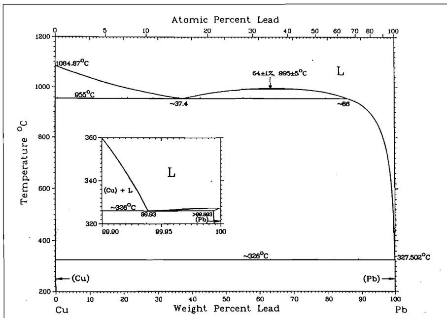
Figure 2: Binary-system Pb-Cu
