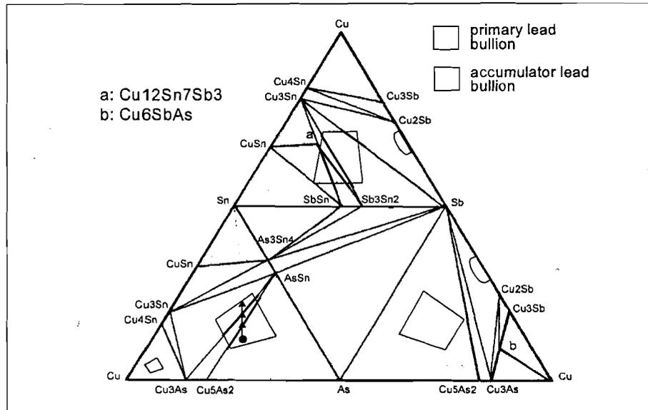
Figure 9: Triangulation of the system Cu-As-Sb-Sn
