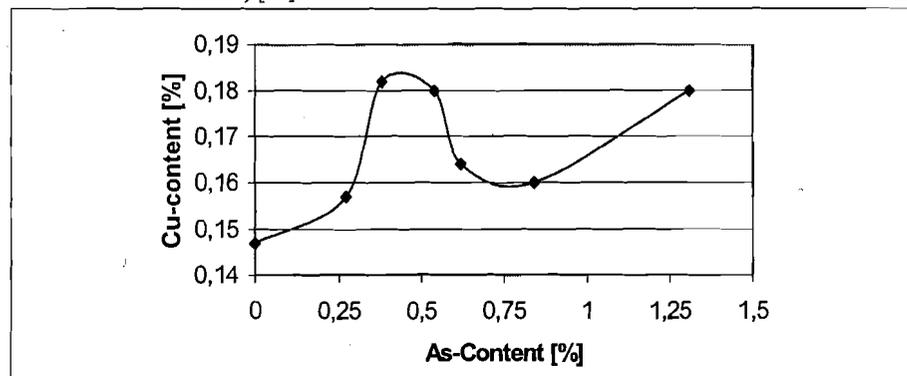
Figure 14: Influence of arsenic on the copper removal in the system Pb-Cu-Sb-As (single sulphur addition 100 %, Cu initial content from 0.30 to 0.50 %, Sb initial content 9 %)
