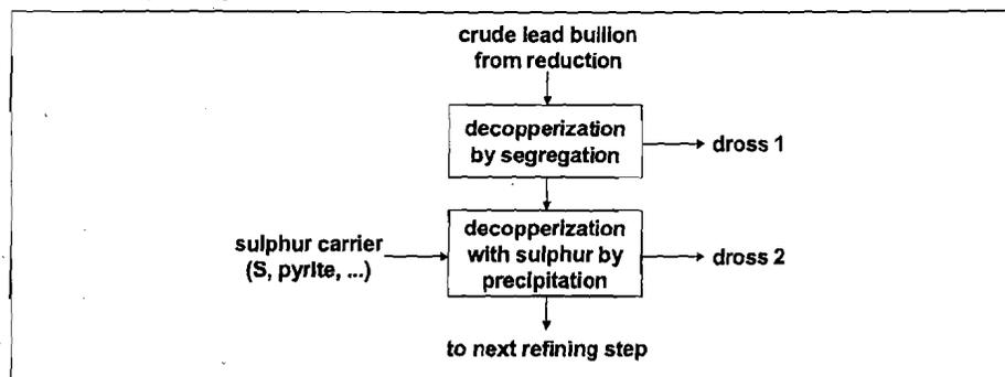
Figure 1: Scheme of the first refining step for crude lead
