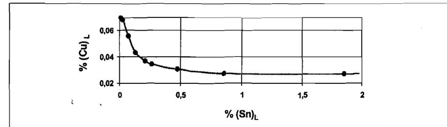
Figure 5: Pb-Cu-Sn-system; isotherm of Cu-solubility at 337 °C
