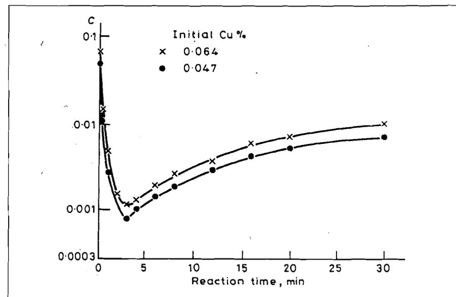
Figure 15: Kinetics of the copper removal from lead with sulphur [40]
