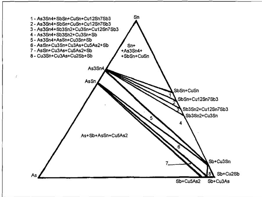
Figure 11: Polythermic cut As-Sn-Sb/Cu = 9,5 (bullion from battery recycling)
