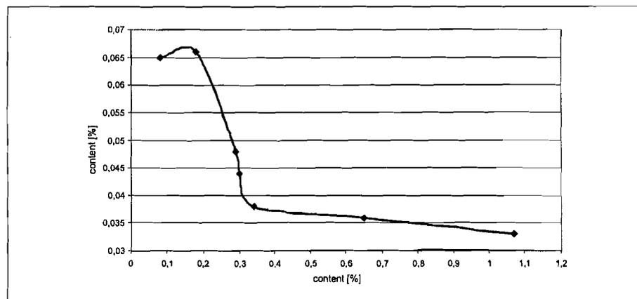
Figure 13: Influence of tin concentration on copper removal in Pb-Cu-Sn-Sn-melts at 285 °C (single sulphur addition 100 % related to  $\text{Cu}_2\text{S}$ , Cu initial content 0.15 to 0.30 %, Sb initial content 9.0 %) [12]
