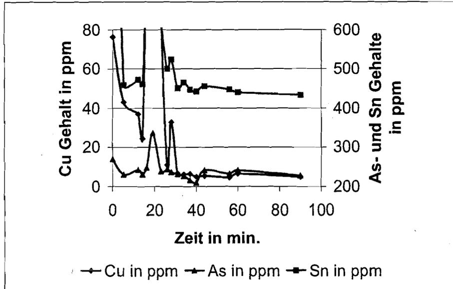
Figure 16: Kinetic curves of copper, tin and arsenic concentration by copper removal in lead with sulphur and pyrite (production samples)
