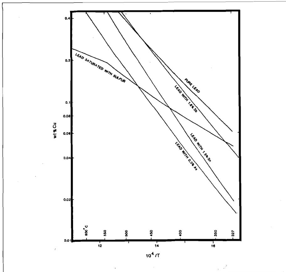
Figure 4: Solubility of copper in lead as a function of temperature in presence of third elements
