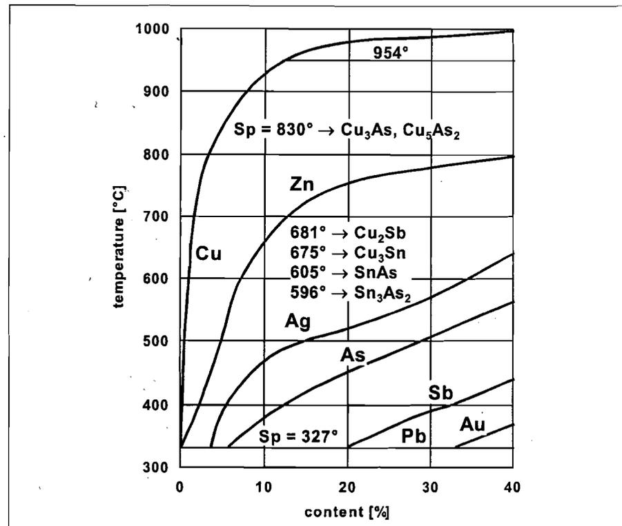
Figure 3: Equilibrium solubility of alloying elements in lead and melting points of relevant intermetallic phases [3]
