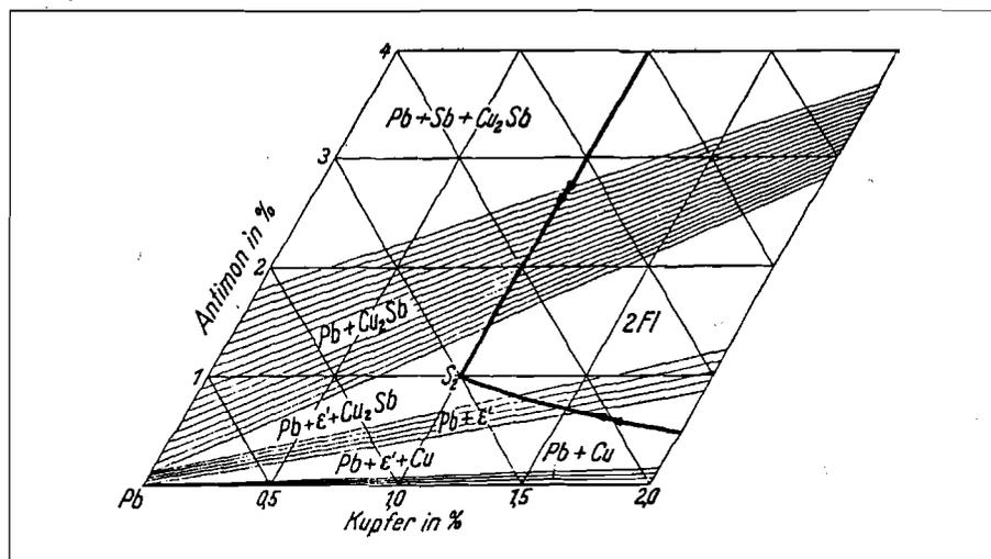
Figure 8: Lead corner at the Pb-Cu-Sb phase diagram after homogenisation at 20 - 30 °C below solidification temperature [11]
