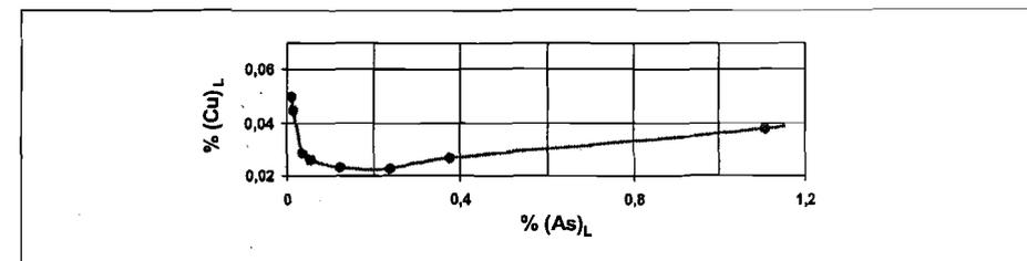
Figure 6: Pb-Cu-As-system; isotherm of Cu-solubility at 337 °C
