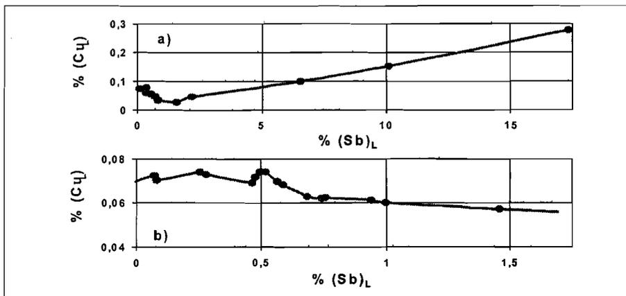
Figure 7: System Pb-Cu-Sb isothermal solubility of copper at 337 °C
