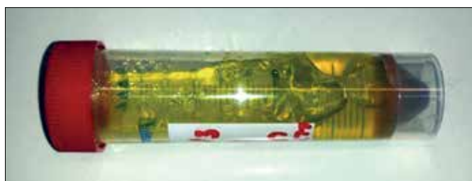
Fig. 3: Silica gel formation in samples during sulfuric acid leaching
