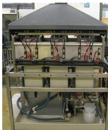
Figure 4 Laboratory Ag electrorefining cells (3 cells in total) at IME Aachen
