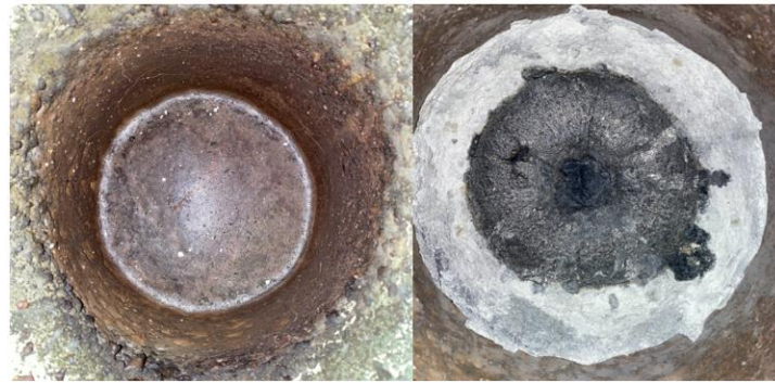
Figure 10: Slag surface and metal of trial Al-Cr-Ti-V (adj.)
