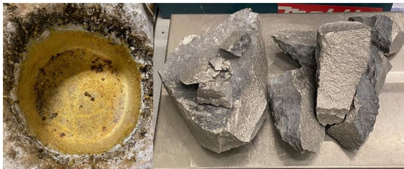
Figure 6: Slag surface and metal of trial Al-Ti-V
