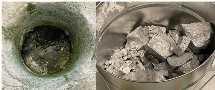
Figure 7: Slag surface and metal of trial Al-Cr-V
