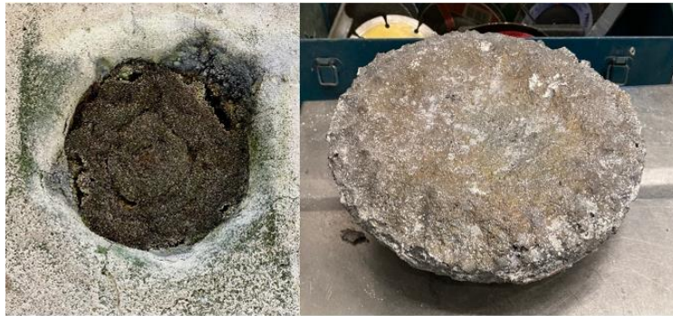
Figure 5: Unreacted top layer and metal ingot of trial Al-Cr-Ti
