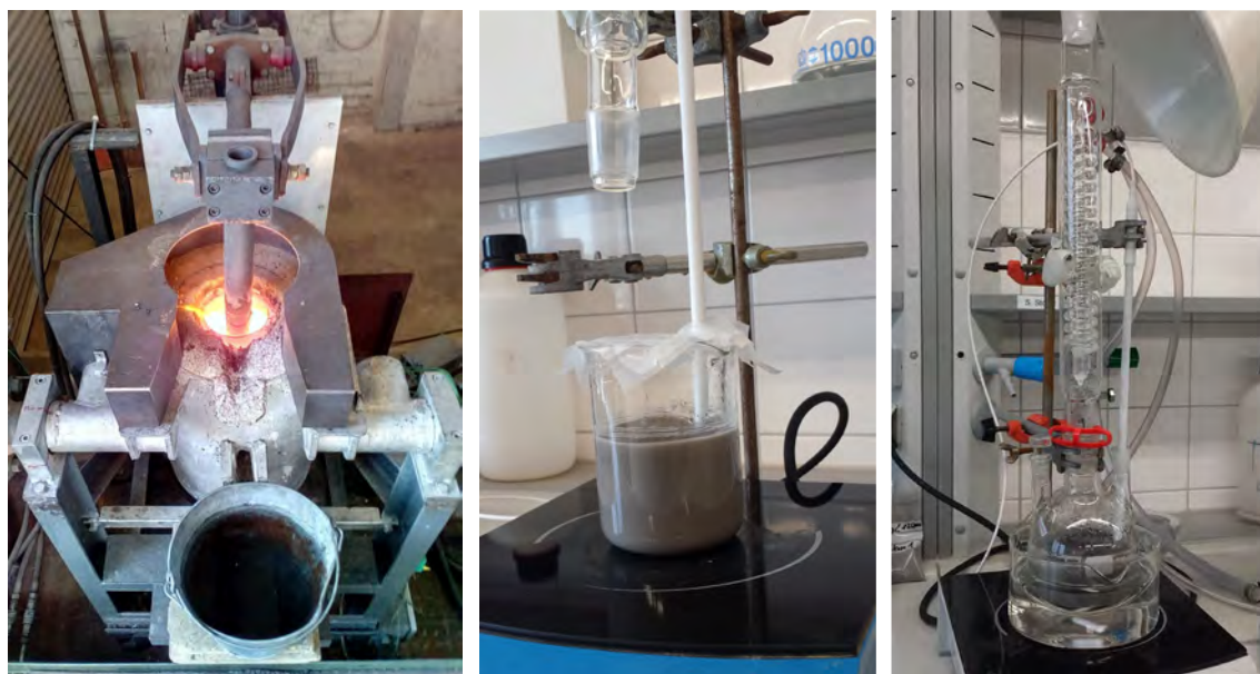
Figure 2. Experimental set-up (from left to right), Electric Arc Furnace, Leaching reactor A, Leaching reactor B.
