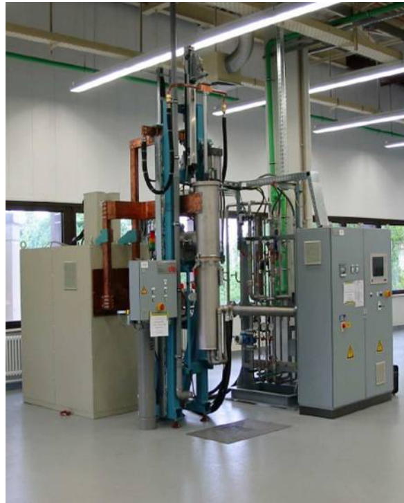
Figure 10: 200kg/200mm vacuum arc furnace to be delivered to the IME in 3rd quarter of 2006
