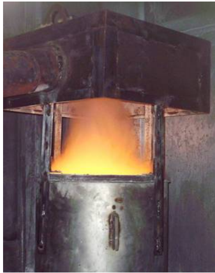
Figure 7: 50 kg laboratory-scale aluminothermic reactor
