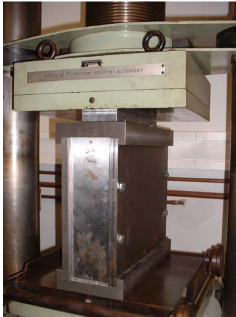
Figure 6: 100 mm die of the 500 t hydraulic press for the compacting of primary VAR and (P)ESR-electrodes from sponge or turnings
