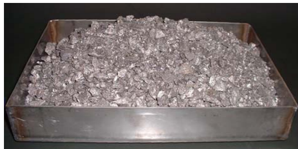
Figure 14: Aluminothermically reduced master alloy after crushing and eddy current separation
