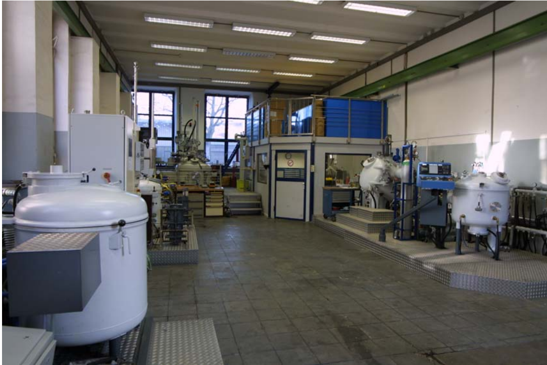
Figure 8: VIM workshop with the 150 kW pilot furnace in the background
