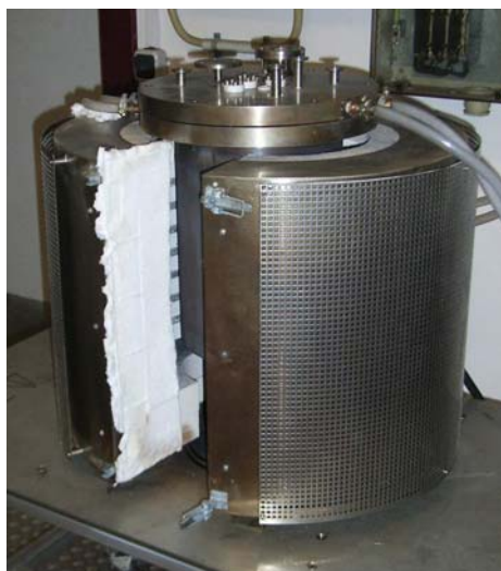
Figure 13: Lab-scale-HDH (hydride-dehydride) furnace
