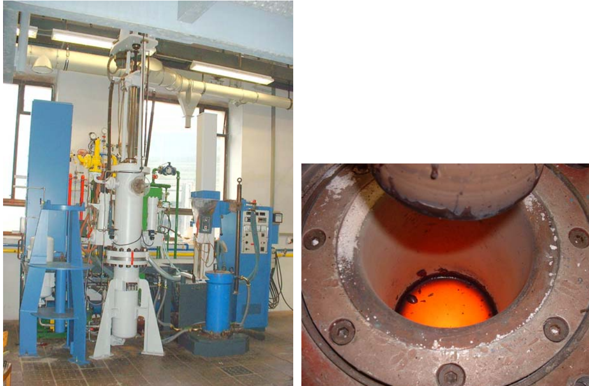
Figure 9: Combined PESR and ESR furnace (left) and detail of the ESR crucible (right)
