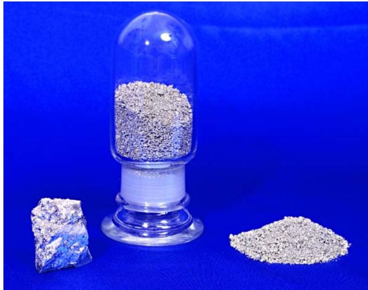
Figure 16: VIM cast (Ti, Zr)Mn 2 hydrogen storage alloy before and after hydrogen embrittlement
