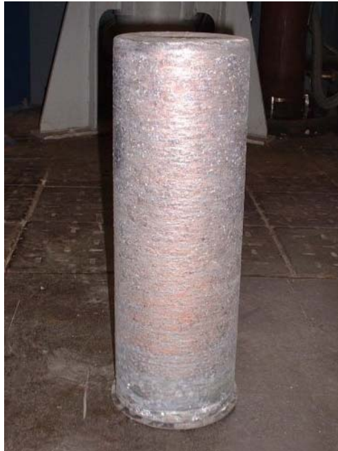
Figure 15: Invar-ingot after VIM-cast and ESR-refining
