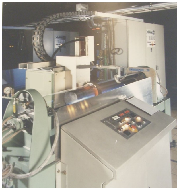
Figure 12: 80 kVA zone refining device for ingot sizes up to 100 mm in diameter
