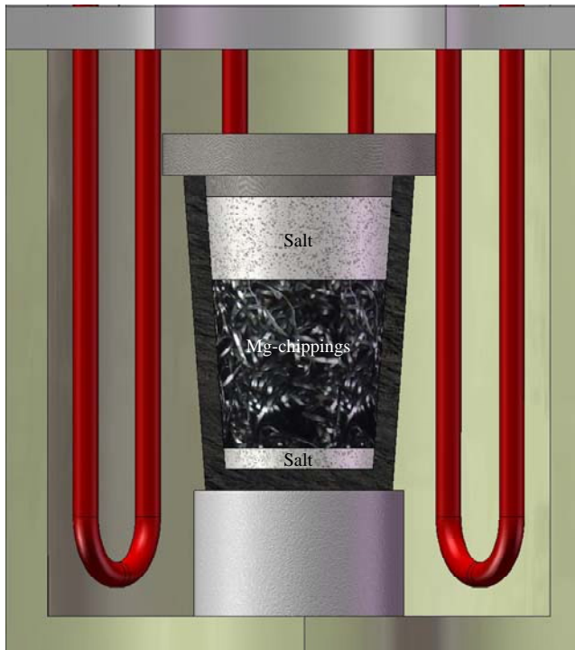
Figure 5: Graphite crucible inside furnace containing magnesium chippings surrounded by two layers of salt mixture and covered up with a refractory lid
