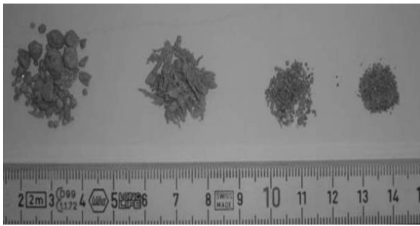
Figure 8: Low-efficiency coagulation of Mg-chippings through salt mixture Nr. 1
