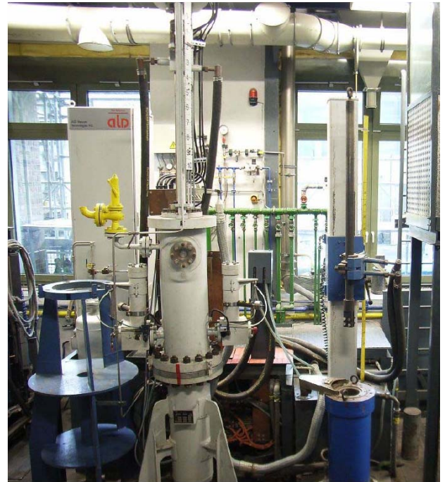
Figure 5: ESR/PESR furnaces at IME Aachen
