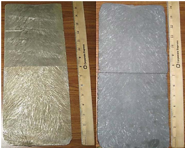
Figure 9: Ingot macrostructure after etching, left: 15-15HS, right: X30CrMoN151
