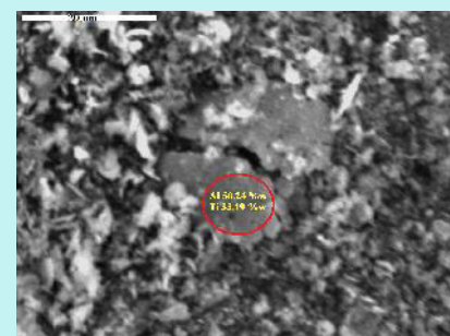
SEM micrographs of GC WE in equimolar melt \text{AlCl}_3 + \text{NaCl} + \text{anodically dissolved Ti} conc. 0.97 at.% Ti; Inserted EDS data of the deposit obtained potentiostatically at -0.400 \text{ V vs. Al} .
