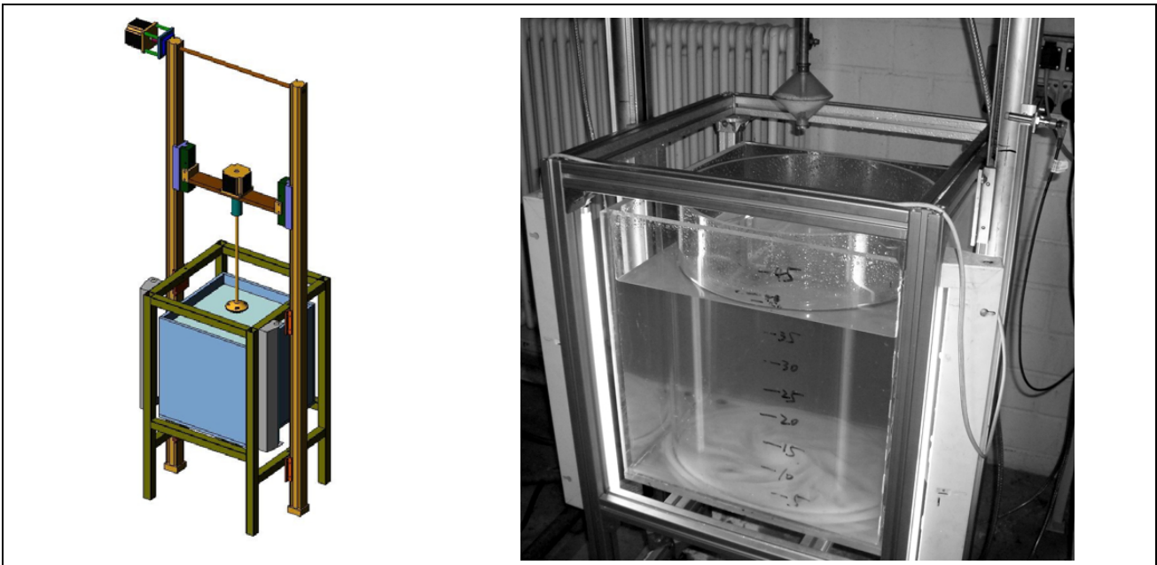
Figure 6: Sketch and picture of the filter centrifuge water model at the IME
