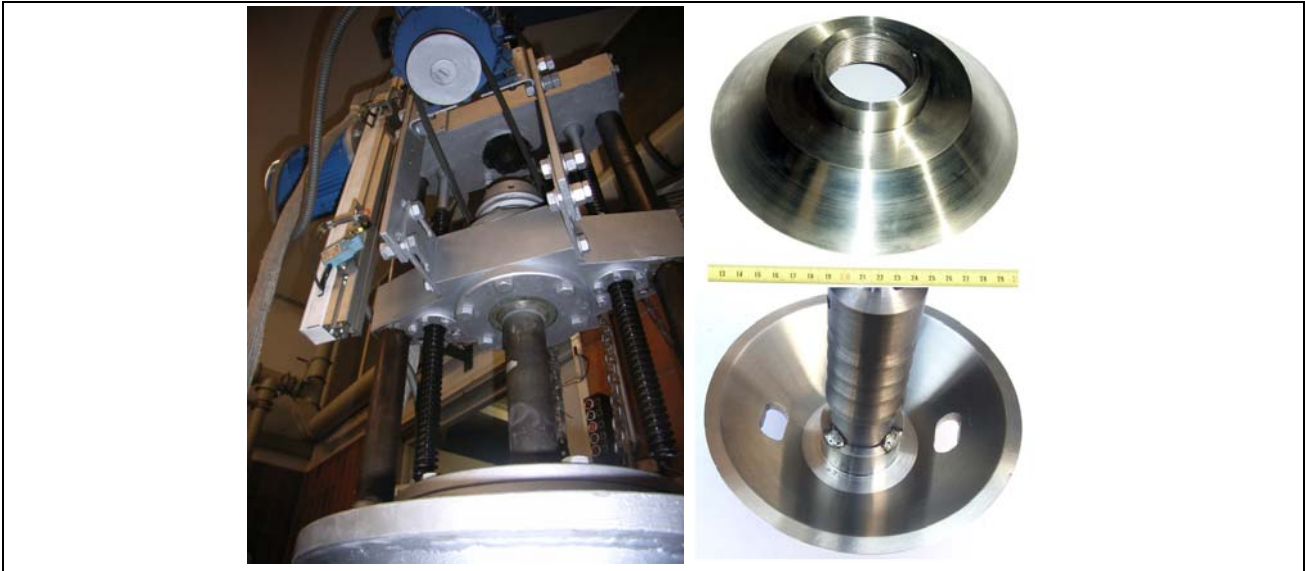
Figure 3: The pilot scale filter centrifuge at the IME (left), cones for separation (right)
