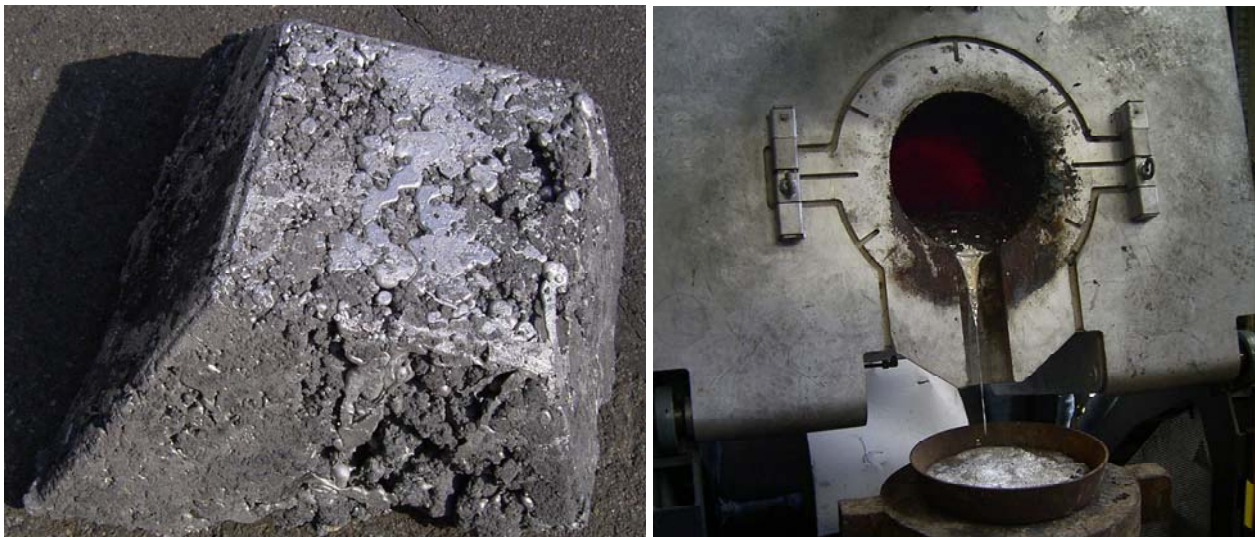
Figure 6: black dross block, separation of metal and sludge
