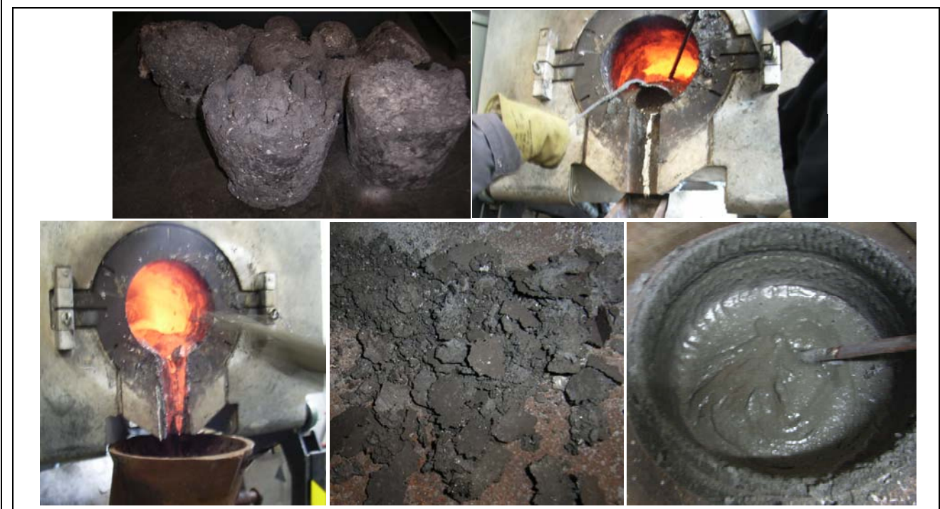
Figure 7: charging material, separation of metal, tapping of hot sludge, filter cake, recycled salt
