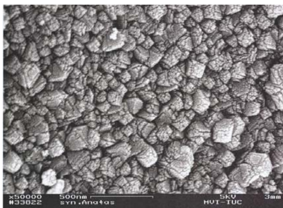
Fig. 9. Scanning electron microscope image of the produced synthetic anatase
