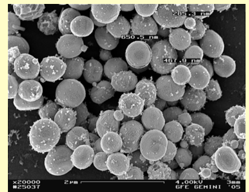
SEM micrograph of Cu-Powder ( T=1000^\circ\text{C} , C_{\text{HCOOH}} = 0.2 \text{ mol/l} )
