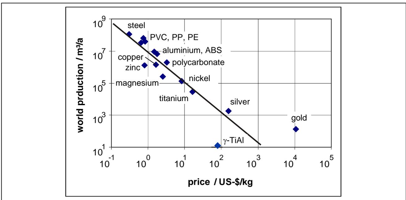
Figure 1: Position of  $\gamma$ -TiAl in the material world (state: 2001 - 2002,  $\gamma$ -TiAl: 2003)
