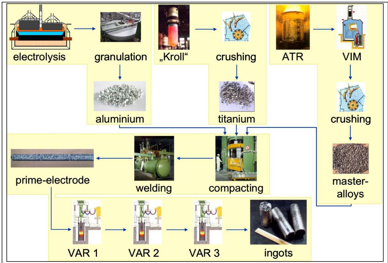
Figure 2: Conventional route for  $\gamma$ -TiAl-alloy production
