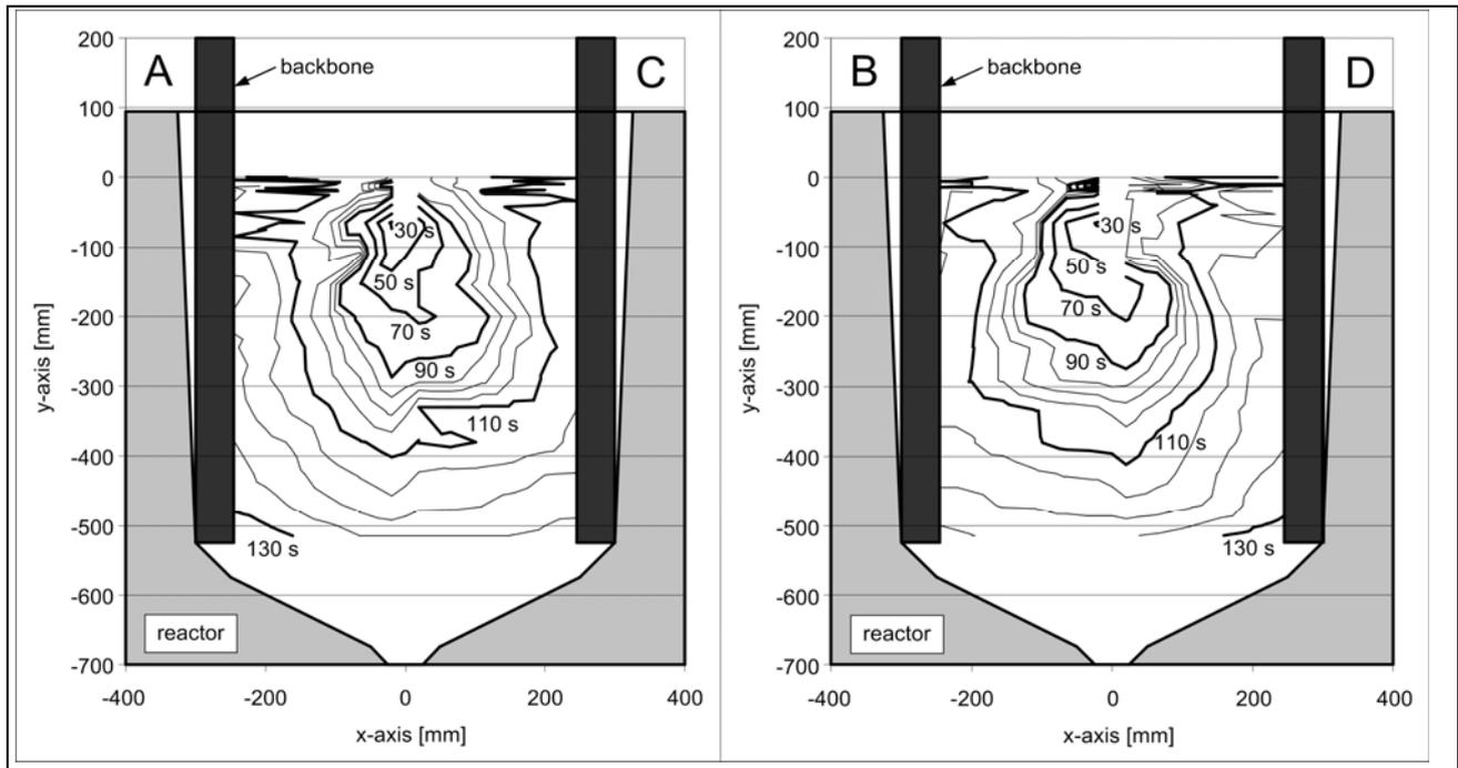
Figure 4: Propagation of the reaction front during the aluminothermic production of a  $\gamma$ -TiAl-Nb-alloy (two cross-sections of the reactor).
