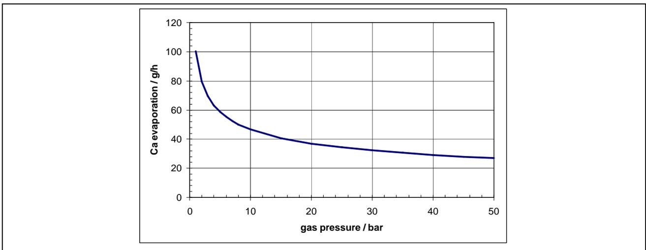
Figure 8: Theoretical Ca evaporation for a 5 wt.-% Ca containing  $\text{CaF}_2$ -slag at  $1720 \text{ }^\circ\text{C}$  ( $\phi_{\text{mould}} = 162,5 \text{ mm}$ ;  $\phi_{\text{electrode}} = 110 \text{ mm}$ ) for increasing Argon pressure in a PESR-furnace
