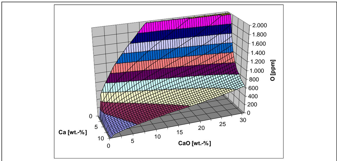
Figure 6: Theoretical oxygen content of a Ti-45Al-10Nb-alloy during electro slag remelting as function of the Ca- and CaO-content in the slag ( $\vartheta = 1\ 600\ ^\circ\text{C}$ , metal in liquid state)
