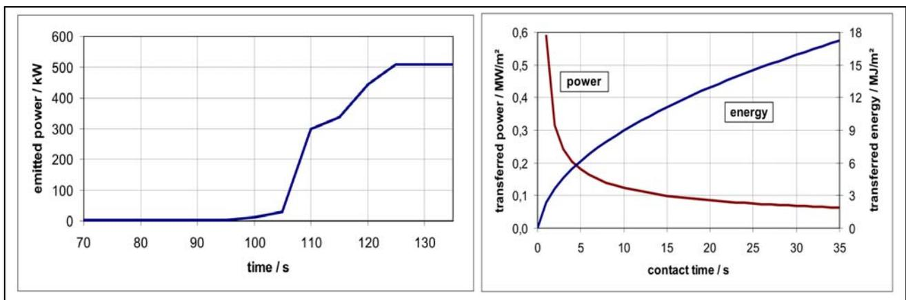
Figure 5: Emitted power losses of the reactor as function of the reaction time (left) and transferred power and total transferred energy as function of the contact time between melt and lining material (right) based on the measurements in [10] and the calculated adiabatic process temperature
