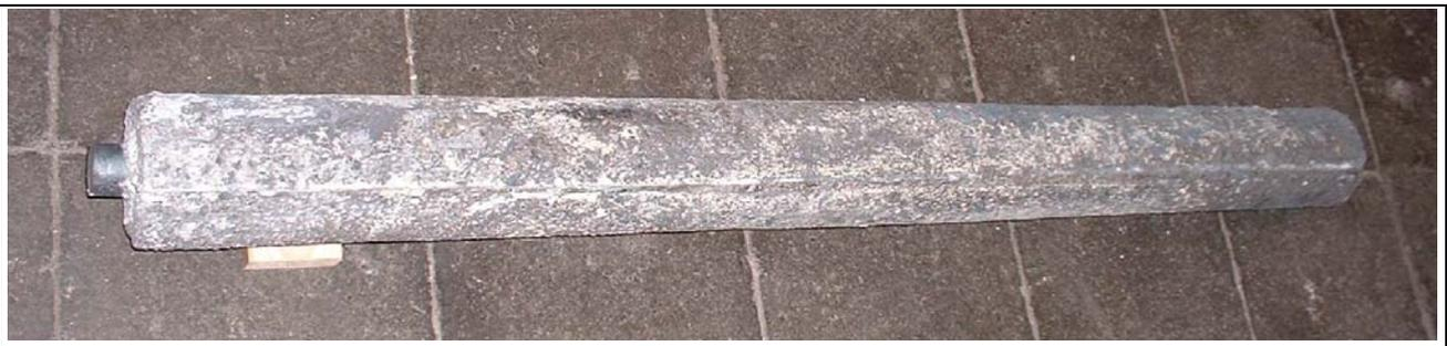
Figure 11: First produced pilot-scale  $\gamma$ -TiAl-Nb prime-electrode (dimensions: 113 x 1 320 mm) with connector for the stub of the electro slag remelting furnace on the left
