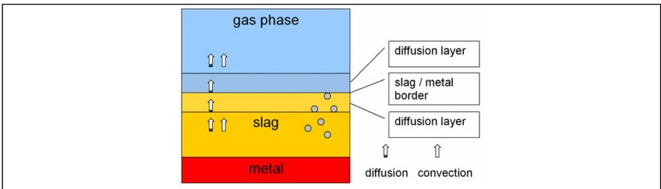
Figure 7: Schematic diagram of the transport layers and transport mechanism for the Ca evaporation (arrows: diffusion/ convection; circles: evaporation)
