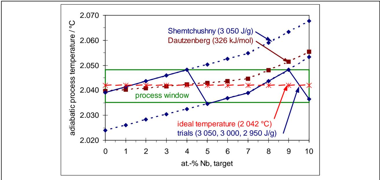
Figure 9: Adiabatic process temperature of the aluminothermic  $\gamma$ -TiAl-Nb production and thermal process window for 20 kg laboratory scale
