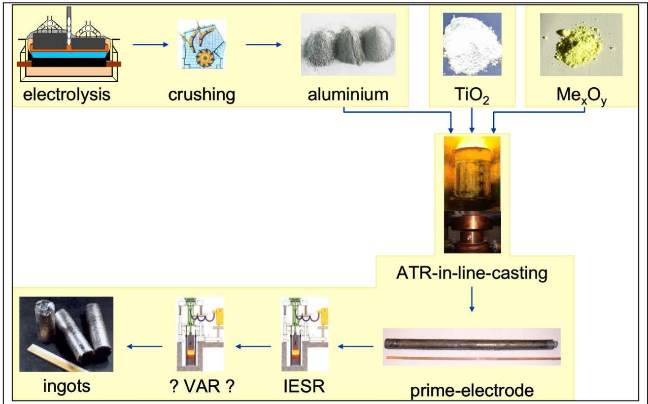
Figure 3: IME process for  $\gamma$ -TiAl-alloy production
