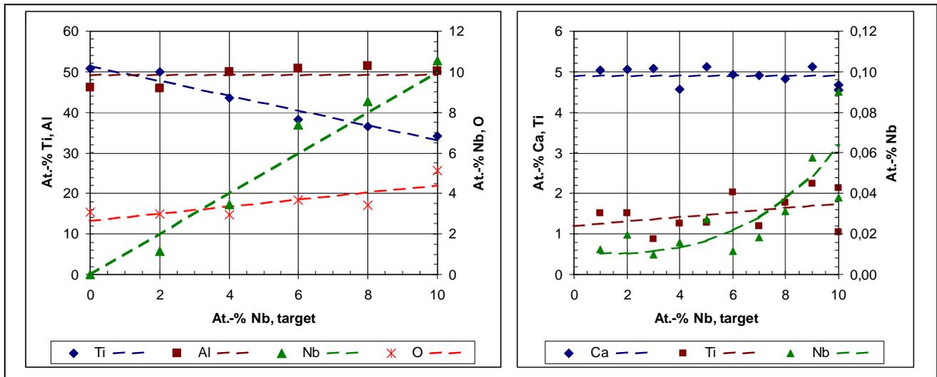
Figure 10: Metal (left) and slag (right) composition of aluminothermic reduced  $\gamma$ -TiAl-Nb
