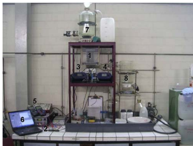
Fig. 3: Electrocoagulation system at IME RWTH-Aachen, Germany
