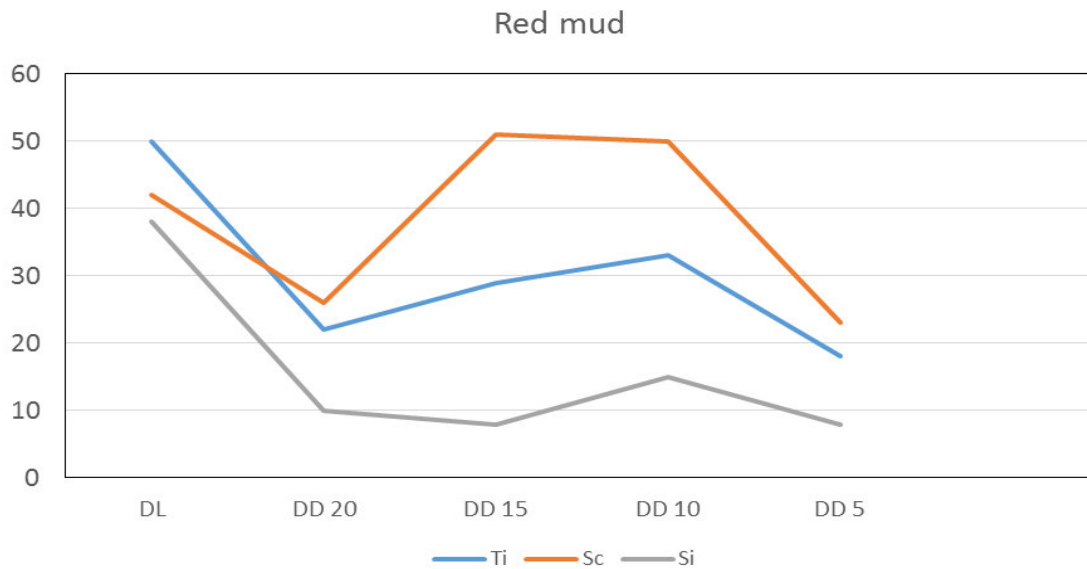
Figure 1. Extraction efficiencies of Ti, Sc, Si from red mud where DL: Direct leaching, DD: Dry digestion
