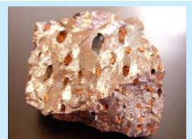
copper-slag: produced matte with Cu-precipitation
