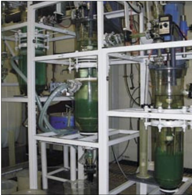
Fig. 6: Detail of the cascade line reactor for continuous neutralization/precipitation
