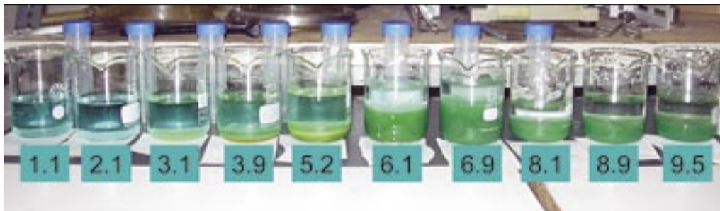
Fig. 8: Consumption of NaOH in all reactors to treat 40 l of synthetic waste water
