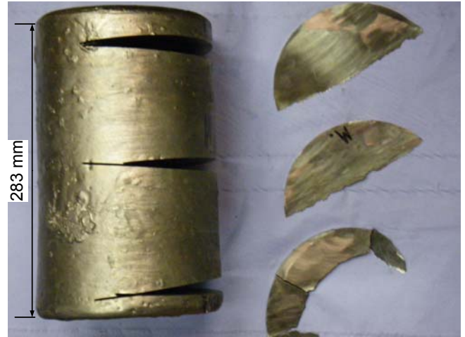
Figure 7: Sampling of obtained, deoxidized PESR ingots
