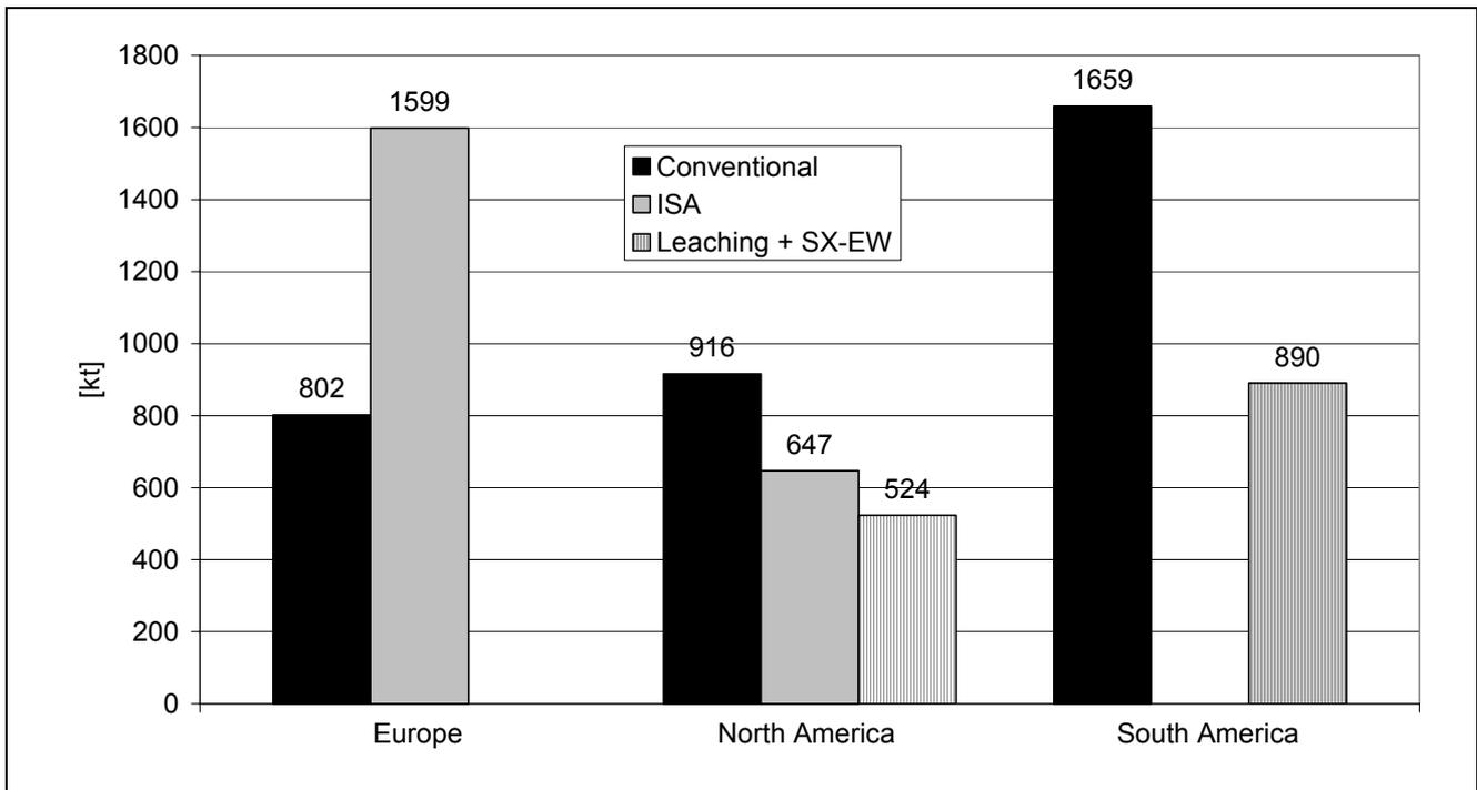
Figure 6: Distribution of electrolytic refining
