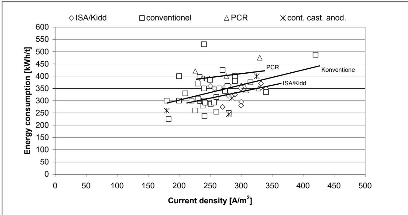
Figure 4: Energy consumption and current density of Copper refining electrolysis
