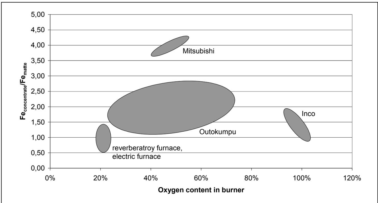
Figure 3: Fe-share of concentrate and matte at ration of oxygen enrichment
