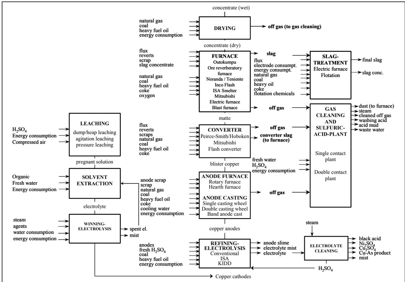
Figure 1: Process chain model of Copper cathode production
