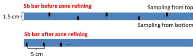
Fig. 5 – Sampling sketch of Sb bar (side view) before and after zone refining.
