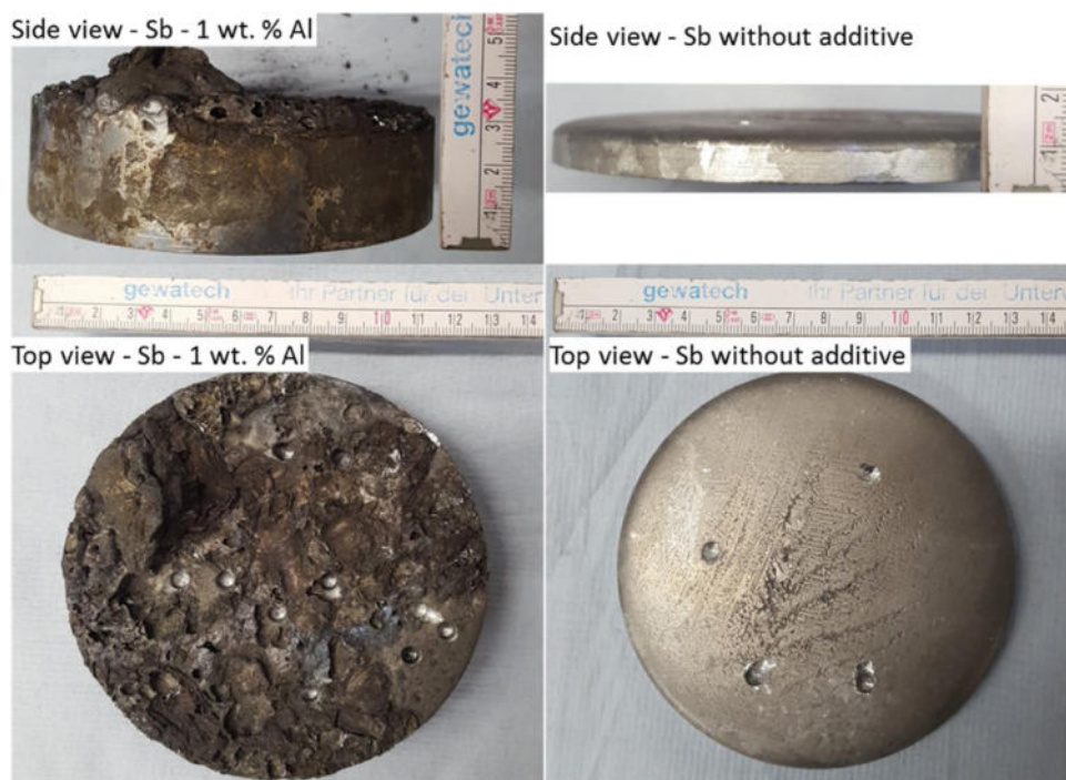
Fig. 9 – Comparison of appearance of residues after vacuum distillation between Sb - 1 wt.% Al (trial No. 9) and Sb without additive (trial No. 8).
