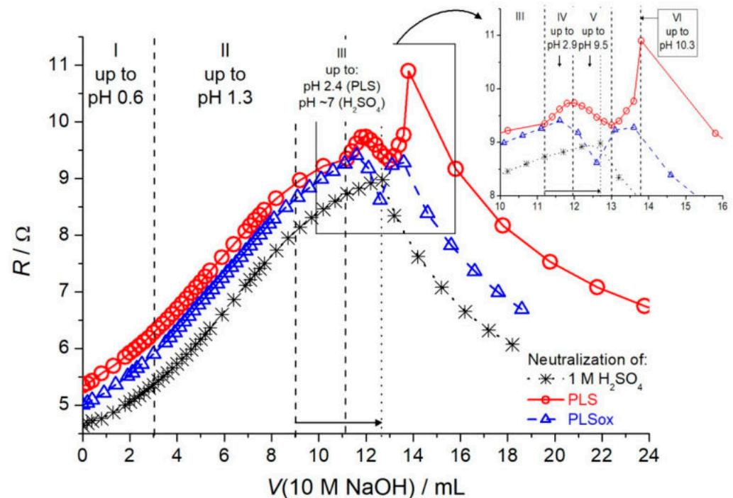
**Figure 2.** The changes in resistance in 1.0 M  $\text{H}_2\text{SO}_4$ , PLS and PLSox upon neutralization by NaOH gained by impedance conductometric measurements. Input voltage: 10 mV r.m.s., 10 kHz;  $22 \pm 1$  °C.
