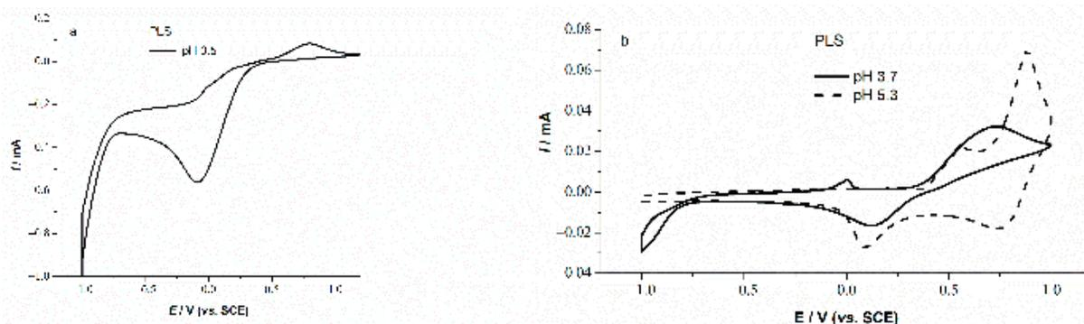
**Figure 4.** Cyclic voltammograms of (a) native PLS at pH 0.5 and (b) NaOH-treated PLSs (pH 3.7 and 5.3),  $v = 10 \text{ mV s}^{-1}$ . The anodic branches are recorded upon hold at the cathodic limit for 2 min.
