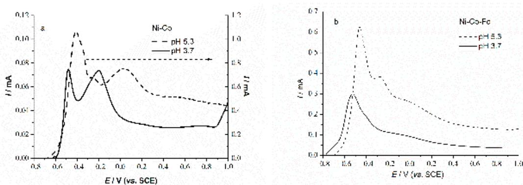
**Figure 8.** LSV curves in phosphate buffer solution (pH 7.2, 25 °C) of deposits obtained after CAs at  $-900$  mV in (a)  $\text{NiSO}_4\text{-CoSO}_4$  and (b)  $\text{NiSO}_4\text{-CoSO}_4\text{-FeSO}_4$ .
