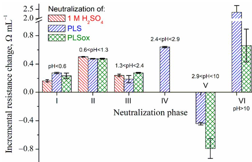
**Figure 3.** The changes in resistance per volume of 10M NaOH added calculated as first derivative of the curves from Figure 2; specific phases of neutralization, I–VI, as well as corresponding pH ranges, are indicated according to intersections of tangent lines. The standard deviations of linearization are presented as error caps.
