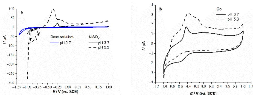
**Figure 5.** CV of GC in  $\text{N}_2$ -saturated (a)  $\text{NiSO}_4$ , compared to base and (b)  $\text{CoSO}_4$  solutions,  $v = 10 \text{ mV/s}$ . The anodic branches are recorded upon hold at the cathodic limit for 2 min.
