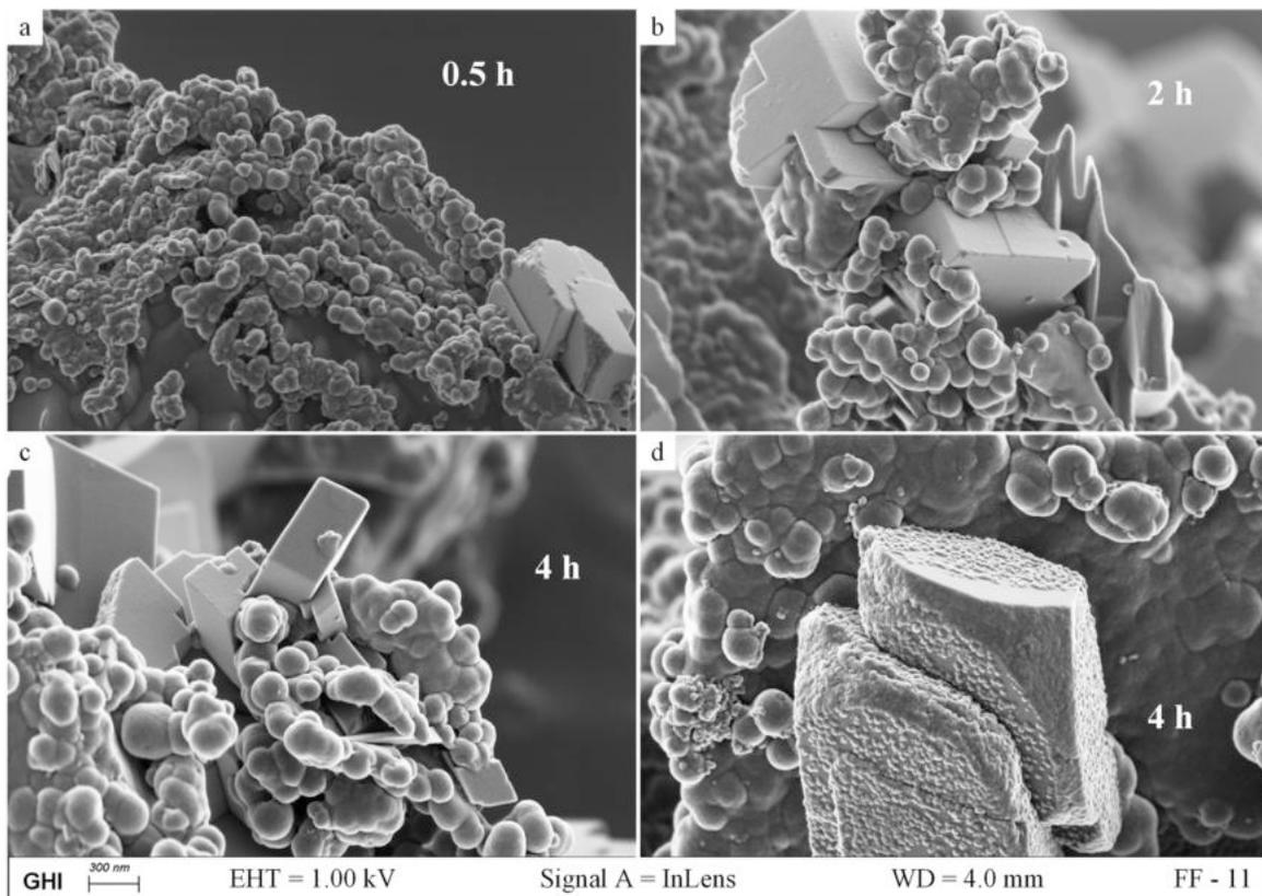
**Fig. 5.** SEM images (30,000 x magnification) of the reaction products sorted according to the retention time. The magnesite particles can be identified by their rhombohedral crystal faces. The amorphous silica is characterised by spherical particles. The magnesite crystals and the amorphous silica are mainly located on the surface of unreacted olivine particles, but are also visible as intergrown particles, which makes subsequent separation challenging.
