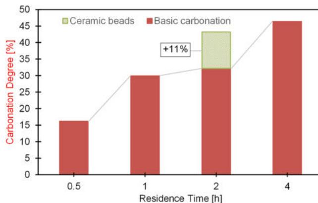
**Fig. 8.** Effect of addition of ceramic beads. The slope in the degree of carbonation is plotted and compared with the different residence times.
