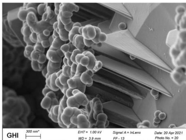
Fig. 9. Amorphous silica particles on the tips of the poorly soluble iron mineral lamellae.
