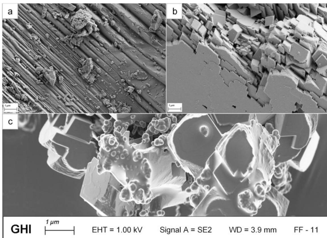
**Fig. 7.** SEM images (10,000 x magnification) of the effect of nucleation with magnesite; (a) unreacted magnesite seed crystal 45 – 63  $\mu\text{m}$ ; (b) Carbonation of olivine < 20  $\mu\text{m}$  with addition of magnesite seed crystals (45 – 63  $\mu\text{m}$ ) at basic parameters – fraction > 45  $\mu\text{m}$ ; (c) Carbonation of olivine < 20  $\mu\text{m}$  with addition of magnesite seed crystals (45 – 63  $\mu\text{m}$ ) at basic parameters – fraction < 20  $\mu\text{m}$ .
