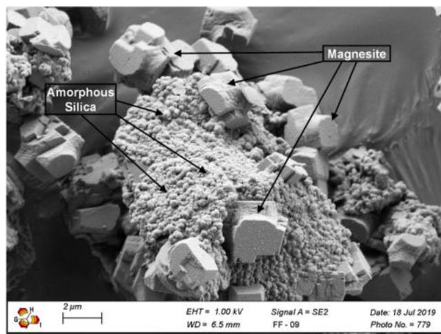
Fig. 2. SEM image of carbonation product for olivine < 20 μm under previously defined basic carbonation conditions. The reaction products magnesite and amorphous silica are indicated [5].
