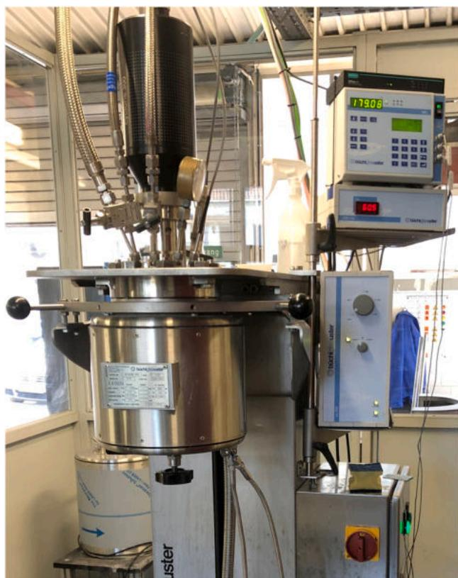
Fig. 1. Büchi Kiloclave in operation.
