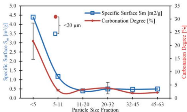
Fig. 3. Effect of differing particle size or specific surface area on carbonation degree. The six consistent particle size fractions are presented and linked in relation to the degree of carbonation and the specific surface area. The fraction < 20 μm is stated separately.
