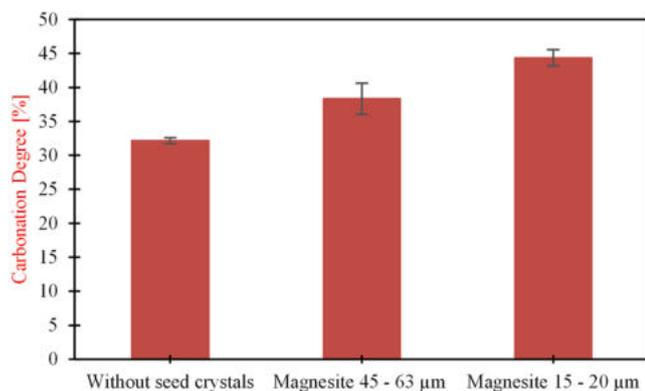
**Fig. 6.** Influence of magnesite seed crystals. The left column presents the carbonation degree at a retention time of 2 h without seed crystals, and the others with the addition of magnesite in two different particle size fractions.
