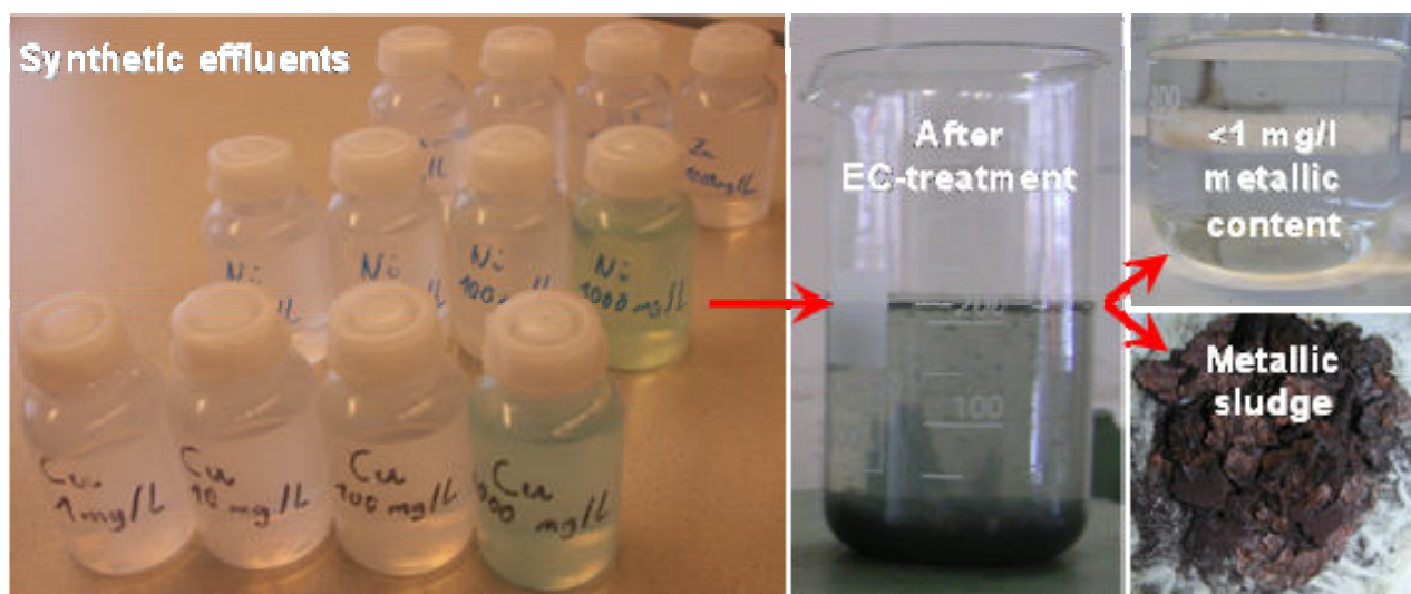
Figure 6: Synthetic and industrial wastewater before and after the electrocoagulation treatment
