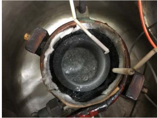
Figure 4. 160 ml graphite crucible with charged feed material
