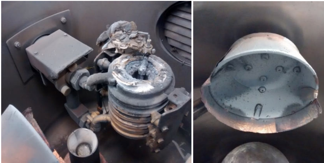
Figure 5. Vacuum induction furnace after trial with AlF_3 -covered copper condenser
