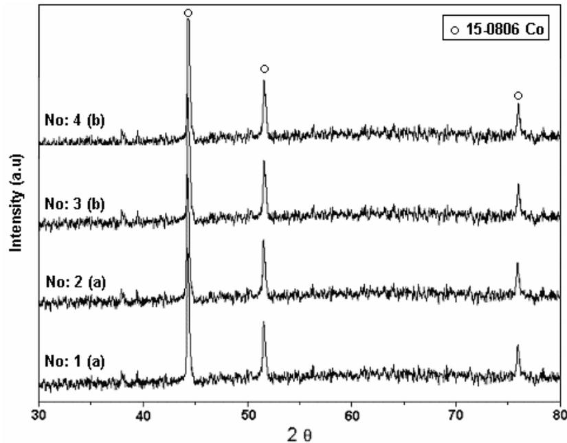
Fig. 6. Typical X-ray analysis of the prepared cobalt powders (800 °C)
