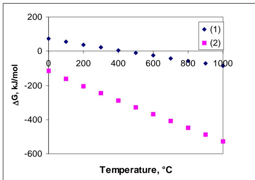
Figure 1. Thermodynamic analysis of hydrogen reduction of  $\text{NiCl}_2$  and  $\text{Co}(\text{NO}_3)_2$
