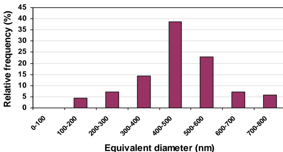
Fig. 9.a. Stereological analysis of Co-Powder prepared by ultrasonic spray pyrolysis (see Fig. 8.a)
