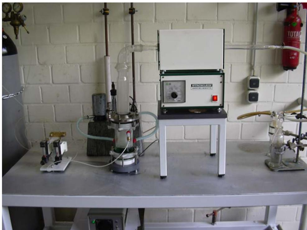
Figure 2. Experimental apparatus for the USP-synthesis of Co/Ni-particles (bottles with  $\text{H}_2$  and  $\text{N}_2$ , flowmeter, thermostate, aerosol generator, quartz tube, tubular furnace, bottles for collection of powders)
