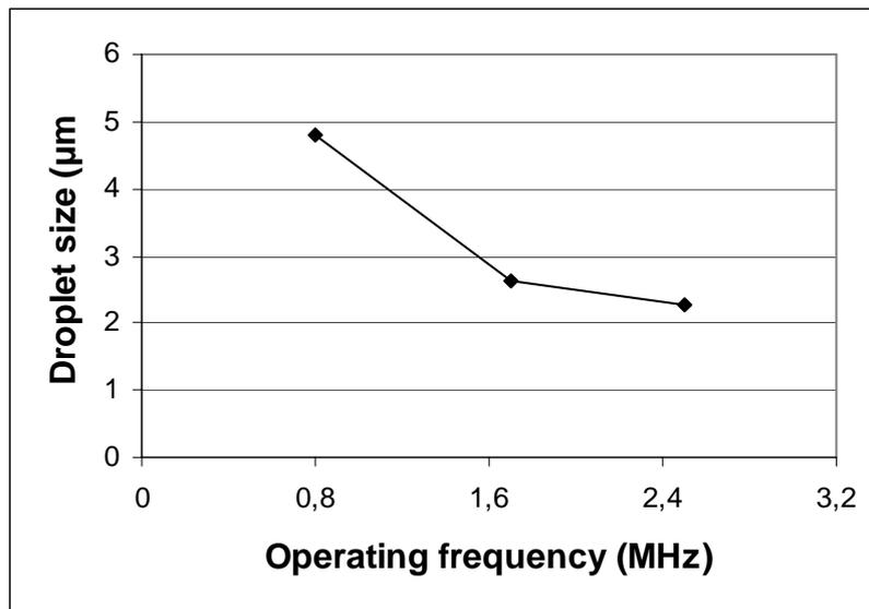
Figure 5. Dependence of aerosol droplet size by the operating frequency
