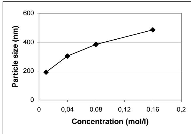
Fig. 7. Calculated values of particle size of cobalt
