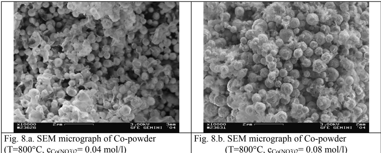
⊕ *Synthesis of particles of Ni- and Co- powders by ultrasonic spray of NiCl<sub>2</sub> and Co(NO<sub>3</sub>)<sub>2</sub> and hydrogen reduction pyrolysis*
