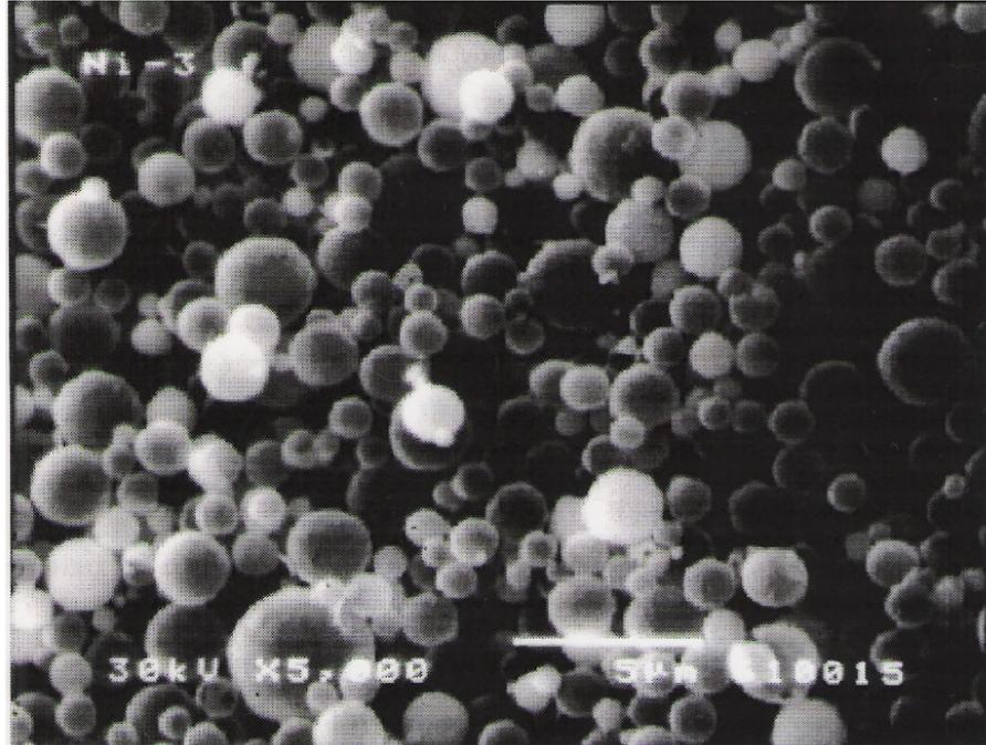
Figure 4.c. SEM micrograph of nickel particle prepared by ultrasonic spray pyrolysis in the presence of 0.1 mass % Pd added
