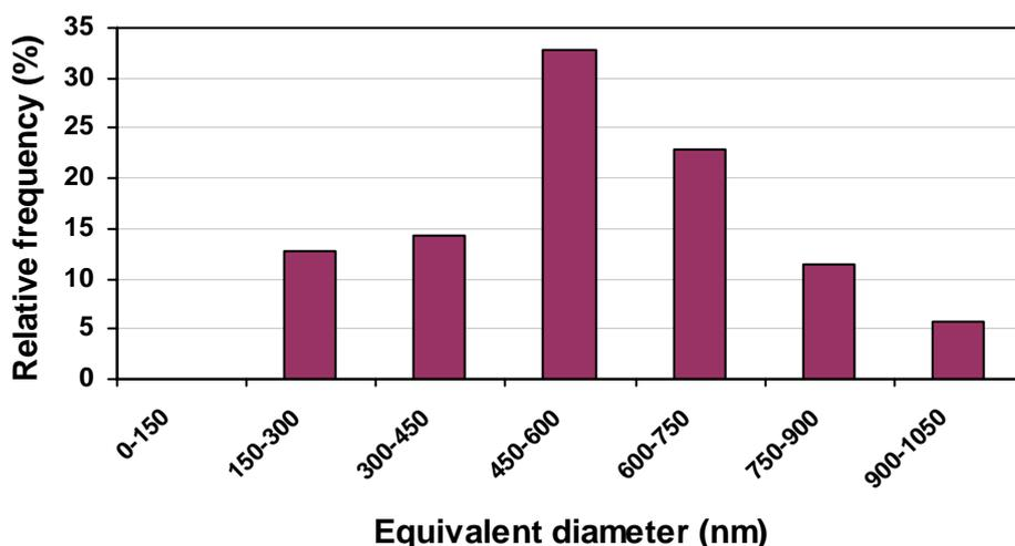
Fig. 9.b. Stereological analysis of Co-Powder prepared by ultrasonic spray pyrolysis (see Fig. 8.b)
