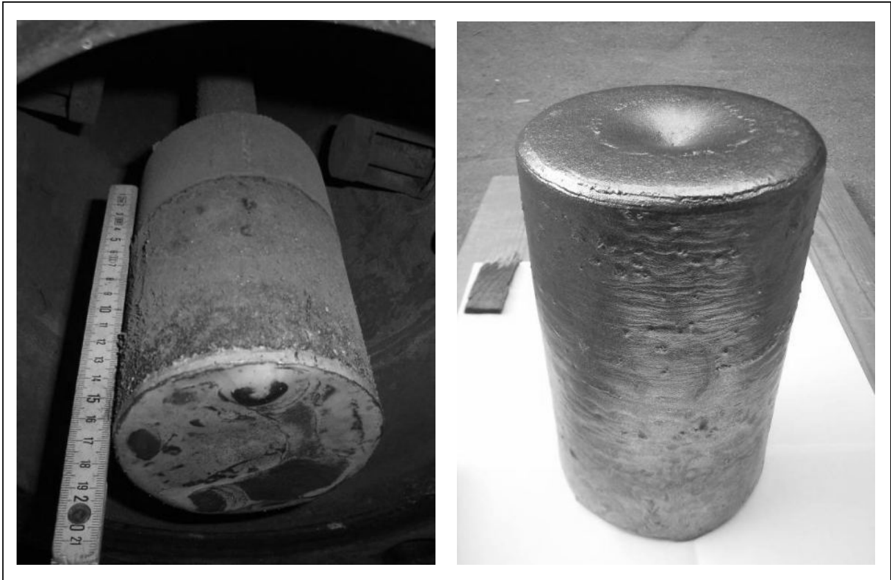
Figure 6: Electrode leftover after PESR with reactive slag and obtained deoxidized TiAl-ingot
